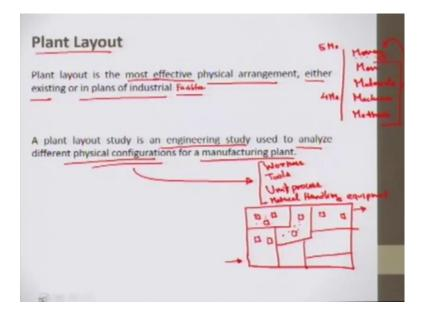
So, how do we define a plant layout plant layout is the most effective physical arrangement either existing or in plans of industrial facilities industrial facilities. So, it has to be most effective how it can be most effective we will see. Now it is arrangement of machines and equipment and it considers certain all the MS of management there are 5 Ms in management, 5 Ms of management are 5 Ms of management are money, men, materials, machines, and methods.
