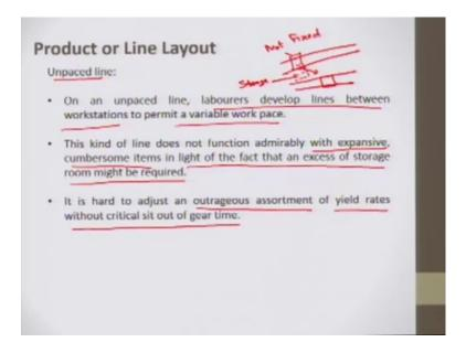
Next is unpaced line in an Unpaced line; the laborers develop lines between workstations to permit variable workplace. So, what happens in unpaced line the product is not fixed on a conveyor it is not fixed, when I use word product here by product I would say my work or my work piece it is not the end product here would have end product or final product.
