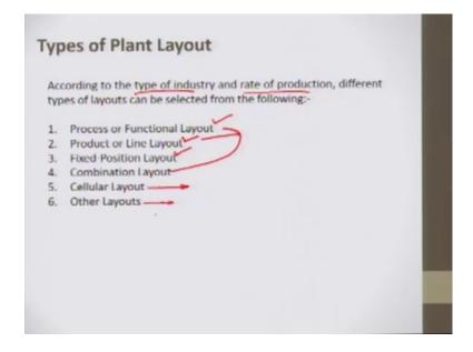
Now, let us come to the types of plant layout. According to the type of industry and rate of production, different types of layouts can be selected from the following number one is process or functional layout, number 2 is product or line layout, number 3 is fixed position layout, then we have combination of these 2 process and product it is known as
