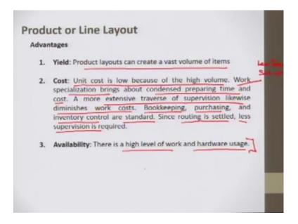
So, say certain advantages of product or line layout the yield or the output the product layouts can create vast volumes of items the yield is too high. The cost the unit cost is low because of the high volume, unit cost is the cost of the product work specializes brings about condensed preparing time and cost preparing time is reduced because there are less setups less frequent setups in here I will put it here.
