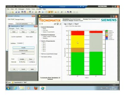
In the report it is telling that there are number of experiment in experiment one, this happened in experiment two, this happened this is the total failure this is both blocked time then grey colour is waiting time, all these things it is telling in the report.
