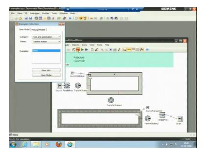
Transfer station is one cell, this 'o' is 1 cell, this is another track here two way track. Transfer station, it will just transfer the material from this cell to this track let me try to see the event simulator, here you can see the trolley or the container came here. The container is coming, some machining is happening at this Parallel Process.
