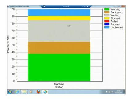
So, for only one machine it is showing the chart that this is something unplanned blue colour is unplanned then we have blocked(yellow), then we do not have any failure here we
