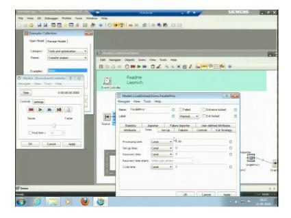
this is a Parallel Process in which 2\*2=4 processes are there and the times is again the default time that is 1 minute. from this source it comes in transfer station, there we need not connect transfer station, when we see a transfer station.
