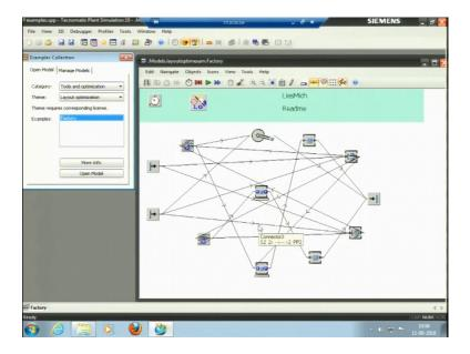
Now layout optimization, factory optimization factory layout is there this is a factory and we have made different kind of connections here. Layout optimization can be done where to keep what machine then what would be the overall, what would there maximum throughput if we do that. So, this can these models can be also we can through these things to find the optimization here.
