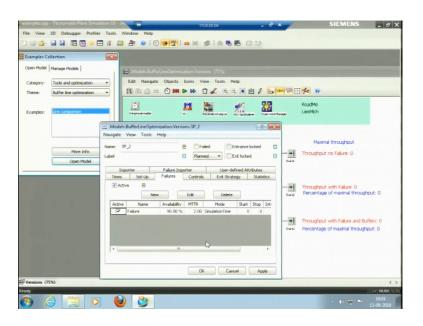
If I see the failure it has 90 percent failure, 90 percent availability, it is 10 percent failure. In this case there is no failure in the first case there is no failure.
