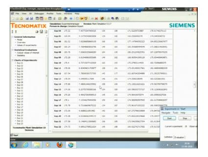
It shows time such as failed time, working time and also it will show the throughput because we asked for a throughput. So, this is the throughput for the 25 experiments so this is the throughput for the 50 observations in experiment number one. Experiment number one means 50 observations that 25 experiments for each experiment there are 50 observations.
