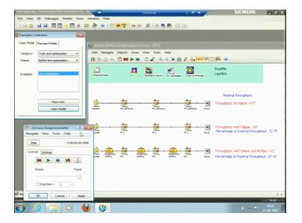
Let me try to run this model yes this model has run for 8 hours a day. For no failure the pieces in a day work for 477 with failure it is 347, but because failure is there we have put the buffers in between that can store some of the material so it is about 417, also it is giving the percentage of the maximum throughput, the maximum throughput is 477, it is with failure we have 72 percent but with buffers it is 7 percent of the throughput of the maximum value.
