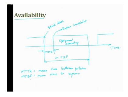
what is MTTR? MTTR is nothing, but mean time between failures and MTBF is nothing, but mean time to repair. And here is the breakdown and here is the repair completed and this is equipment in operation.
