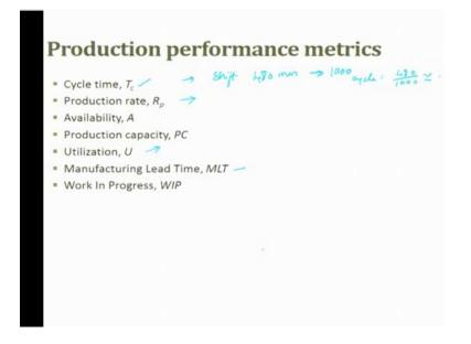
**Production performance metrics:** talks about cycle time, how do you calculate the cycle time? For example, if in a shift there are 480 minutes of working and if it has to produce 1000 items. So, the cycle time is nothing, but 480 minutes by 1000 and this is
