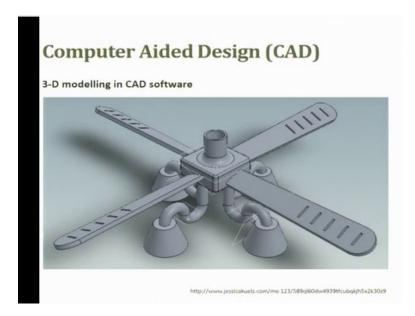
This is a 3-D model, CAD software product. You can see these are the parts or the subassemblies whatever it is, but here you do not get to see the dimensions, you do not get to see the assembly inside the part. So, these are 3 D model in CAD software's which tries to give us the overall impression, but you do not get much of dimensional and assembly informations.
