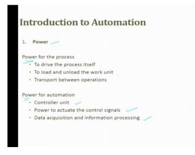
The power for the process is to drive the process itself, to load and unload the work unit, to transport between operations is the powers job. Power for automation is control unit, power to actuate and data acquisition and information processing.
