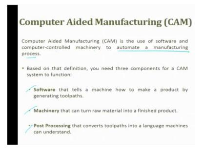
CAM is a software and computer control machinery to automate a manufacturing process. Based on the definition you need 3 components for CAD software, machinery and post processing. Software tries to tell the machine how to work on the product, machinery processes the raw material into finished product; post processing converts the tool part into a language machine understanding.
