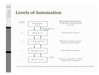
The flow of data happens here, corporate information system is enterprise, production system is plant, manufacturing system group of machines is cell, individual machines is machine level, devices, sensor, actuators and other hardwares
