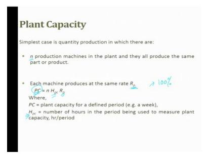
The simplest way of calculating the plant capacity is quantity production in which there are n production machines in a plant and they all produce the same part or product So, each machine produces at a rate of  $R_{p}$ . So, *PC* plant capacity is n products are produced in  $H_{pc}$  into  $R_{p}$ . What is  $H_{pc}$ ? Number of hours in the period during which used to measure the plant capacity ,hours per period, with this we are trying to calculate the plant capacity.
