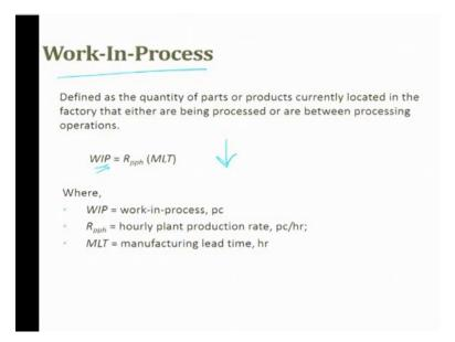
What is WIP? WIP is defined as the quantity of part or products currently located in the factory that either are being processed or are between processing operation is called
