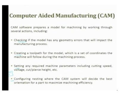
The CAM software prepares a model for machining by working through a several actions including checking if the model has any geometrical error, creating a tool part of the model, setting any required machine parameters and configuring listing, when the CAM system will decide the best orientation for a part to maximize the efficiency.
