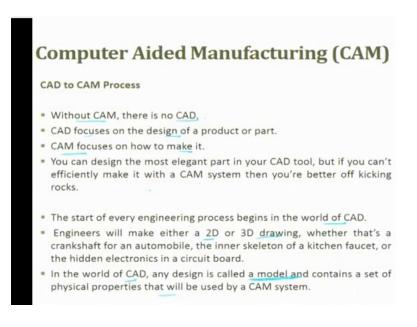
CAD to CAM process without CAM there is no CAD, the CAD focuses on design of a product CAM focuses on how it is to be made. You can design the most elegant part in
