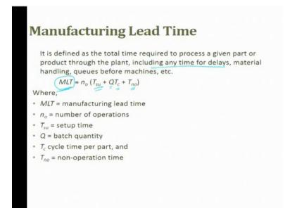
what is manufacturing lead time? It is defined as the total time required to process a given part or a product through the plant, including any time for delay, material handling, queues before the machines, etc.
