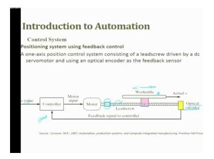
The control system can also be used for positioning. So, here is a system in which the position is controlled .Here is a feedback control system which is used in a CNC machine, the values are given, the controller gives the value to the motor and the motor actuates, there is a coupling.
