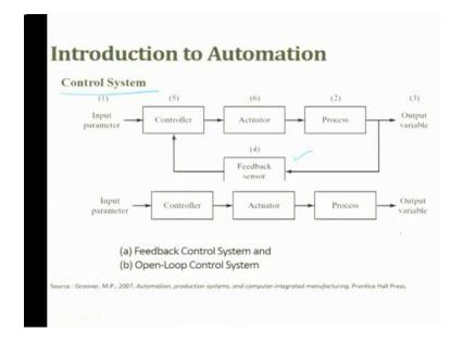
As the input parameter we have controller, actuator, processor. If, there is no feedback it is called as a open loop system, if there is a feedback, it is called as a closed loop system.
