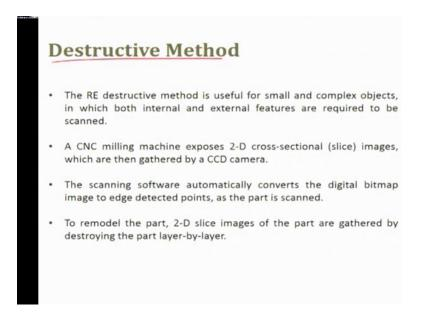
We will next see the destructive methods, destructive method is useful for small and complex objects, with which both internal and external features can be scanned.
