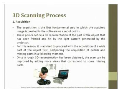
Acquisition: acquisition is the first fundamental step in which the acquired image is created in the software as a set of points. These points define a 3D representation of the
