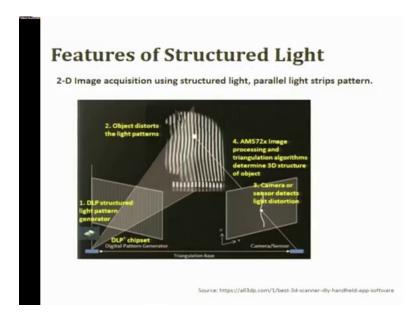
You can see a DLP structure, light pattern is generated, the light goes from here and then DLP is generated, then the object distorts the light pattern, the object distorts the light
