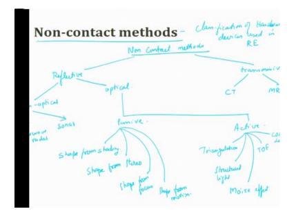
**Non-contact methods:** can be on reflective or it can be on transmitive. CT and MRI are also non-contact techniques in which we try to get the data, in reflective type again you can have non optical or optical.
