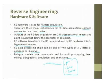
**Reverse engineering hardware and software:** when we talk about reverse engineering hardware and software, RE hardware is used for the RE data acquisition. There are three major technologies for RE data acquisition one is
