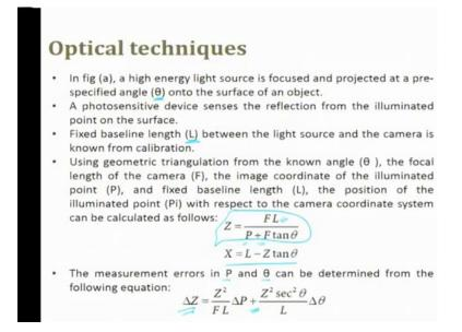
So, from figure a the high energy light source is focused on and projected at a pre specified angle  $\theta$  onto the surface, the photo device senses the reflection from the illumination point of surface, the fixed base length is L. Finally, if you look at it you get through the formula of this where is at the geometric triangulation from the known angle
