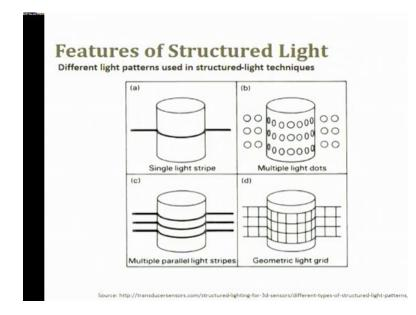
These are the different types of structured light, a single light strip then multiple light dots, multiple parallel light strips, geometric light grids. These are projected and then the details are collected.
