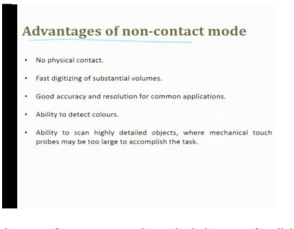
What is the advantage of non-contact type?, no physical contact, fast digitization of sustainable volume, good accuracy and resolution for common applications, ability to detect colour can be done, ability to scan highly detailed objects where mechanical touch is not possible, all these places we go for non-contact type coordinate measuring machine or non-contact techniques.
