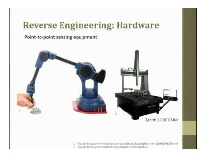
This is a point to point(P2P) sensing system, this is CNC-CMM system, the probe touches and is not electrified. It is only a physical touch you try to measure and it is a trigger probe the other one is also the same, it (P2P) has a frame in which the arm is used, here(in CNC/CMM) arm is not used, a gantry is used. So, the geometry is different the structure is different, but the data whatever you get is a point data.
