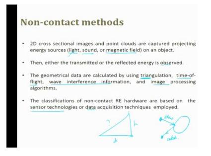
The next one is non-contact type method, here we use a 2D cross section image or a point cloud are captured, projecting an energy source like light, sound or magnetic field.
