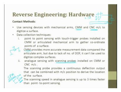
contact type used sensing devices with mechanical arm, CMM and CNC machine to digitize a surface.
