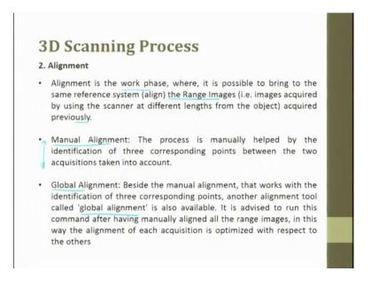
**Alignment:** alignment is a work phase where it is possible to bring to the same reference system, the range images (acquired previously), for example if I have an object placed in a plane and suppose if the object is slightly deviated then there would be an error.
