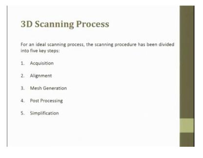
In a 3D scanning process, for an ideal 3D scanning process the scanning procedure has been divided into acquisition of data, alignment of data, mesh generation, post processing and simplification. These are the five steps which are involved in 3D scanning process. Suppose if it is not aligned in one particular plane, it is misaligned. So, alignment can be a problem.
