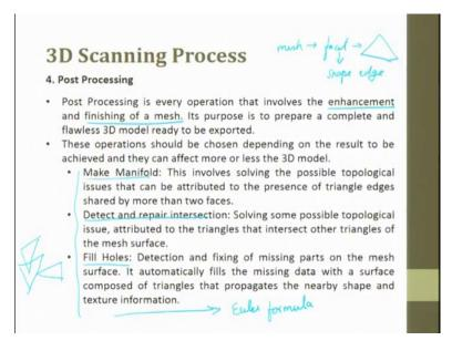
Then comes the post processing: post processing is every population that involves the enhancement and finishing of the mesh.
