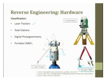
When we talk about hardware, there are four different types of hardwares. one is called as the laser tracer in this system where and which it can swing around this plane and this can swing around this and the height can be adjusted. The next one is a total station.
