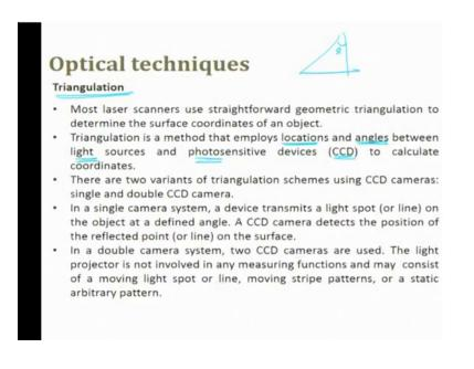
The technique which is used in optical, most common is triangulation, most laser scanners use first straightforward geometric triangulation to determine the surface coordinates of an object.
