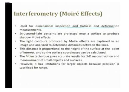
Moiré fringe patterns or interferometer used for dimensional inspection and flats and deformation patterns, we use Moire fringe patterns, We use Michelson's interferometer, which is used to measure the angular displacements that's what they are structured like pattern, are projected on a surface to produce a shadow Moire effect.
