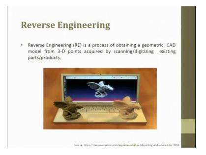
What is definition for reverse engineering? the reverse engineering is a process of obtaining a geometric CAD model from 3D points, acquired by scanning/digitizing existing parts/product. For example You look at a product and try to take a photo of the product or you try to replace that image/photo which was taken through the light now through a laser.
