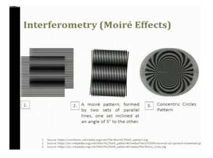
This is a typical Moire fringe pattern. A Moire fringe pattern form a two sets of line which is angled at 5 degrees, this is a concentric circle pattern which is made. You keeps growing and when you try to take the image of it from the image you can try to correlate and try to find out the 3D object.
