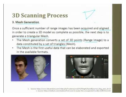
Once you made the point data, the point data is assembled and you try to do a mesh generation, once a sufficient number of range images have been acquired and aligned, in order to create a 3D model as a complete as possible the next step is to triangulate the mesh.
