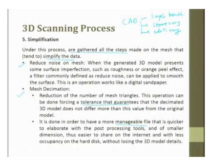
The last thing is simplification: under this process, are gathered all steps made on the mesh that tends to simplify the data.
