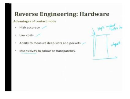
The accuracy of contact measurement, is highly accurate, it is low cost, ability to measure deep slots -you wanted to do high aspect ratio holes then contact measurement is the only way, insensitivity to colour or transparency is removed from here.
