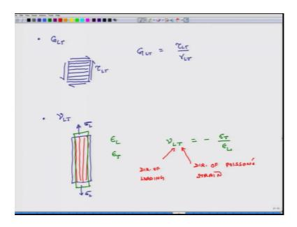
G L T and how do you measure G L T? You take a sample and you subjected to some shear test shear stresses. So, this you can do either on a rectangular slab, but it can be more easily done on pipes and you can subject them to torsion, so that is much more easy to.
