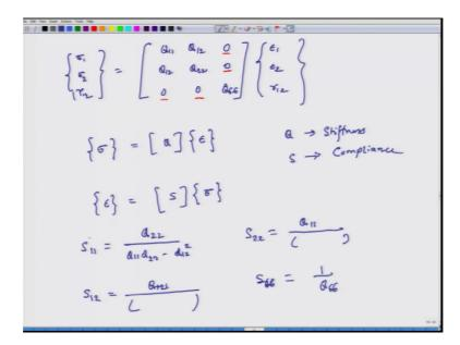
So, sigma 1, sigma 2 and tow 1 2 and the strain vector through the stiffness matrix Q; so this would be epsilon 1, epsilon 2, gamma 1 2 and we have Q 11, Q 12, 0 Q 12, Q 22 0, 0, 0, Q 66.
