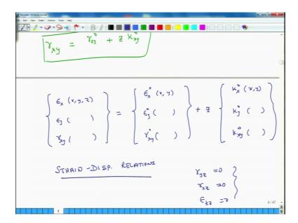
So, I can say that epsilon x epsilon y gamma x y and all these are functions of x y and z. These are equal to their mid plane components; epsilon x evaluated at mid plane, epsilon y evaluated at mid plane and gamma x y evaluated at mid plane plus the value of z coordinate times mid plane curvatures k x naught again evaluated mid plane k y naught
