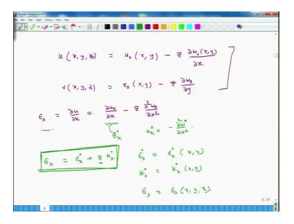
So, the relation which we had developed was u which can vary. So, it is u which is a function of x and y and z is nothing but u naught which is the mid plane displacement minus z times delta partial derivative of w and w is a function of x and y. So, it is because it is being calculated or measured at mid plane. So, partial derivative of w naught with respect to x. So, this is the relation for u.
