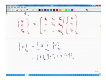
So, we will put a subscript k; this is equal to; so, for each layer there will be a Q bar matrix there will be a Q bar matrix. So, it will have Q 1 1 bar Q 1 2 bar Q 1 6 bar Q 2 2 bar Q 2 6 bar and Q 66 bar and then these are all this is a symmetric matrix.
