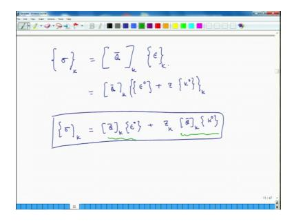
So, I can write sigma for kth layer is Q bar matrix for kth layer times the mid plane strain vector plus z for kth layer because curvature is again independent of layers times Q bar matrix for kth layer times curvature at the mid plane. So, this relation will help us calculate strain stresses at any point in a given layer. So, what do I do? Suppose, there is a particular point in a given layer, first step is that I find out its value of z based on our coordinate system.
