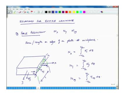
So, what we will develop now is we will start developing relations at the plate level. We, till so far we have been just been talking about the stress strain relations at the level of a particular layer. Now, before we start developing this we will introduce two terminologies one is called force resultant, and there are 3 types of force resultants N x, N y and N xy. So, what is a force resultant? It is force per unit length on edge of a plate. So, add the mid plane, this is important.
