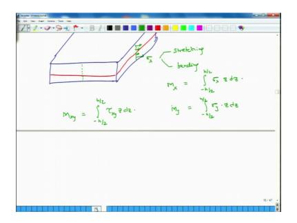
So, to understand how much the plate is going to experience the bending moment we will define a term moment resultant M x. And what is M x? M x is integral of minus h by 2 to h by 2 sigma x, z d z. This is the moment experienced by the plate in the x direction per unit length per unit length, and.
