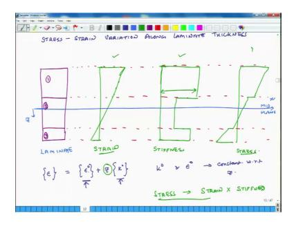
So, the first point of today's agenda is the stress strain variation along laminate thickness, ok. So, let us consider a laminate and for purposes of simplicity we will just make a laminate which has 3 layers. So, this is layer number 1, layer number 2 and layer number 3, so the top layer second layer and the bottom layer.
