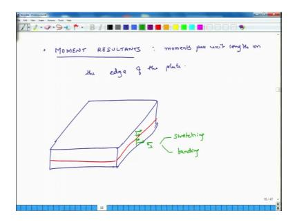
So, this is the other term we should understand before we start developing relations between at the plate level, so moment resultants, ok. So, these are moments per unit length on the edge of the plate, ok. So, let us understand what these mean.
