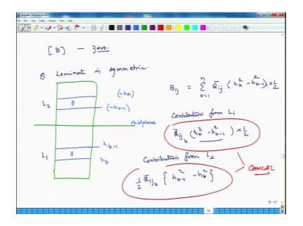
The next thing we discuss is to ensure that the B matrix is0 the B matrix is 0 and to ensure that what we have to make sure is that the laminate is symmetric. If the laminate is symmetric then all values in the B matrix they will come out to be 0 why does this happen?
