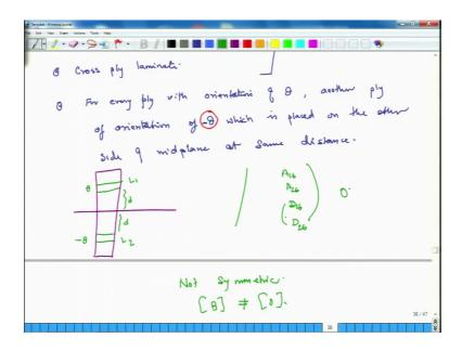
So, what it means is that suppose I have a laminate this is the mid plane and this is a ply of orientation theta and let us say this distance is d.
