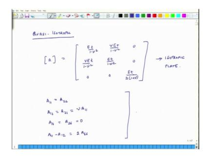
So, these quasi-isotropic laminates they are such that they are isotropic in the plane of the laminate. If you go out of the plane they may still be anisotropic, but within the plane wave behave as isotropic laminates; which means that there A matrix because, A matrix relates to stress stresses and strains within the plane of the plate.
