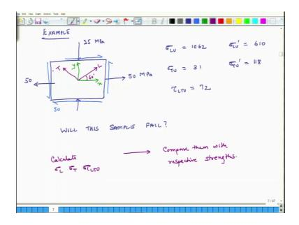
So, consider an example where we have a piece of composite, actually it is just a single layer of orthotropic material and the layer is such. So, this is my x axis, this is y and then my fibers are in this direction.
