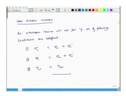
So, the first theory we will discuss is Maximum Stress Theory. So, what does it say? It says that a composite, an orthotropic lamina will not fail if all of the following conditions are satisfied. So, what are these conditions? So, if you have an orthotropic lamina which is loaded the first thing you have to do is, you have to find out what are the values of sigma L, sigma T and tau L T and then you look at these conditions.
