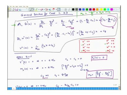
So, which means that minus q x square over 2 plus C 3 x plus C 4 is equal to 0 at what? x is equal to plus minus a over 2 ok. So, if we implemented these boundary conditions what we find is that C 3 is equal to 0 and C 4 is equal to q a square over 8. So, anyway; so, this is one solution for V and for the relation for M works out to be M x is equal to q a square over 8 minus q x square over 2; so, this is the relation for M x ok.
