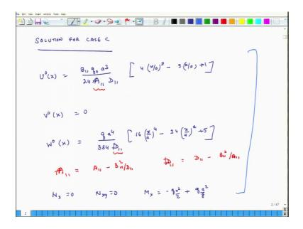
So, the solution for case C; we will just recap the solution for case C by solving the differential equations; it was U naught of x equals B 11, q naught a cube and a is the length of the plate; this is the length of the plate is a and just to recap the coordinate system is located at the center.
