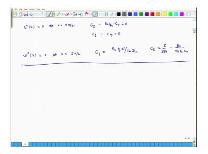
So, what it means is that C 5 minus B 11 over A 11 times C 7 is equal to 0 ok. And that can and the other thing which comes out is that C 5 is equal to C 7 is equal to 0. So, this is what you get and then we when we implement the conditions on W which is W naught is equal to 0 at x is equal to plus minus a over 2; we can calculate the value of C 8 and C 6.
