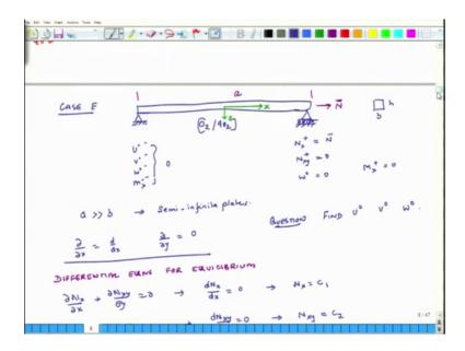
So, let us look at the definition of the problem so, let us call it case E and here we have a plate which is fixed at one end, I mean pinned at one end, but the pin connection is not rolling. So, it is fixed and the other end is on rollers so, this is the plate. The lamination sequence of the plate is 0 to 92 so, 0 layer is on the top and then, we have 90 degree less on the bottom and then, this plate is being subjected to N x at this edge.
