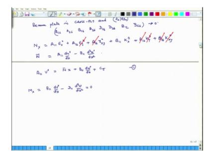
And before we do that we note that because plate is cross ply and 0 to 92 a lot of terms in A B D mattresses are 0. What are these terms? A16 A26 B16 B26 D16, D26 B12 and B66, all these terms are 0, because it is a cross ply laminate ok. This is important B12 and B66 is also 0 for cross ply.
