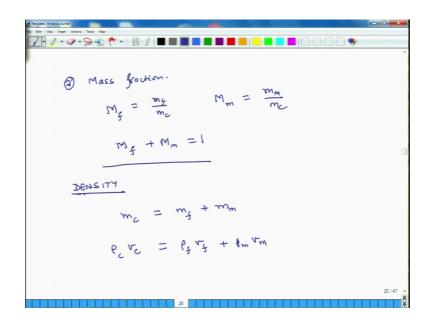
The second terms is mass fraction, this is not that often used but it is still a useful entity to entity and the definitions are similar, So, mass fraction of fibre is mass of fibre divided by mass of composite, mass fraction of matrix equals mass of matrix divided by mass of composite and then of course, the mass of air is almost 0 so we ignore it.
