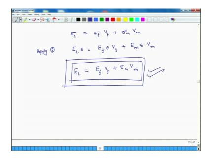
And using these 2 assumptions and principles of linear elasticity, we were able to come to this expression for E L, which is Young's module which is the modulus of the composite in the L direction.
