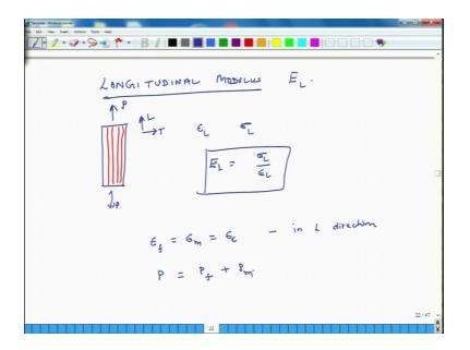
The next parameter we will discuss will be longitudinal modulus. And we designate longitudinal modulus as E L. So, physically what does it mean? What it means is; that if I have a composite material and this composite material is a single layer, reinforced with
