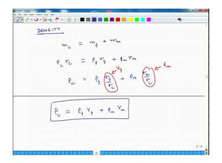
And I divide this entire expression by V c. So, I get density of the composite material equals rho f V f over V c plus rho m V m over V c, but V f over V c is volume fraction of fibre and this is volume fraction of matrix. So, my expression for composite is rho c equals rho f V f plus rho m V m. So, that is my expression for composite material density.
