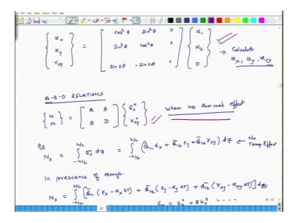
The next set of changes which we had discussed, and before we go to the next set of changes. How do we calculate alpha x and alpha y, gamma x y, it is if alpha 1 and alpha 2 which are the coefficients of thermal expansion in 1 and 2 directions of the material, they are known, then we can compute alpha x, alpha y, and gamma x y through these relations. So, we can calculate that.
