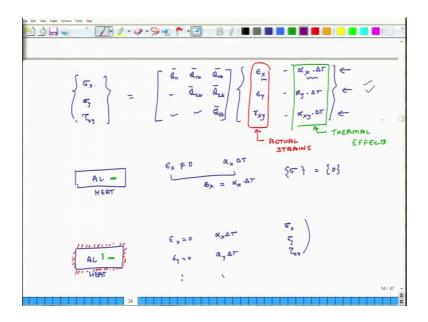
And then we made these relations more general, and we said that sigma x, sigma y, tau x y are related to the strains from based on these relations. And here the important thing to remember is that epsilon x, epsilon y, and gamma x y, they are the actual strains, which we may be able to measure, if by putting strain gauges, so their actual physical measurable strains. While alpha x, alpha y, and alpha x y times delta T, they are mathematical entities.
