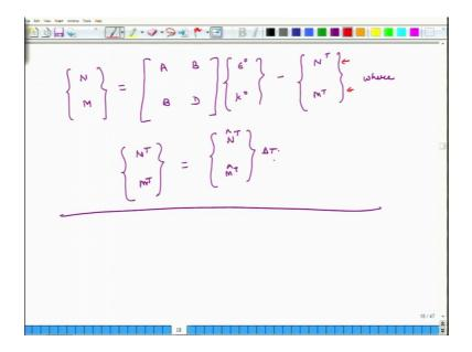
But the moment we have thermal effects the relations between N, M and mid plane strain and mid plane curvatures, they get modified. And these are the modified relations, which account for thermal effects so, this is there. And to recap, so what we have is two additional terms N T and m T. And these and terms N T and m T are account for the temperature effects, and they are nothing but multiples of N T and hat T and delta T, and M hat T and delta T.
