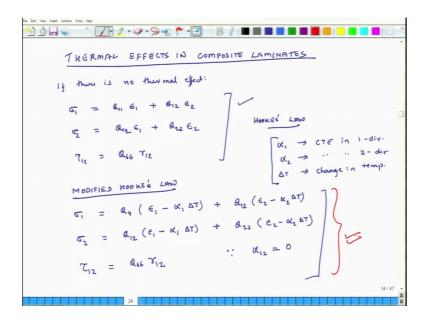
So, the first modification we did was that if there is thermal effect, then the Hooke's law relations which are these, they get modified to these side sort of relations. And here alpha 1 and alpha 2 are coefficient of thermal expansions of the material in 1 and 2 directions. And these modified relations relate stresses to strains in the system.
