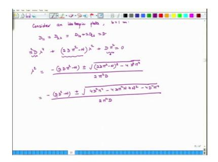
So now, we will consider the case consider an isotropic plate and which is 1 meters in width so, 1 meter wide. So, for an isotropic material we have shown earlier that D 1 1 is
