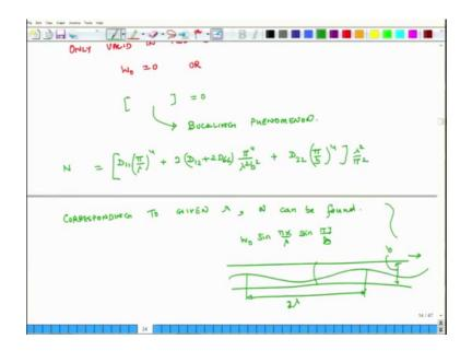
So, this is one condition or this term in green brackets, this becomes 0 and that condition corresponds to the buckling phenomena. So, either w is 0 or W can be non 0, but the term in the green brackets that has to be 0.
