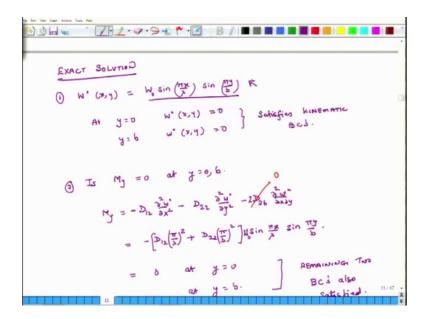
What we had also done was that, we had assume that displacement function for w between displacement out of plane in the out of plane direction and we have seen that if we use this kind of a function than this function satisfies all the boundary conditions associated with the infinitely long simply supported plate.
