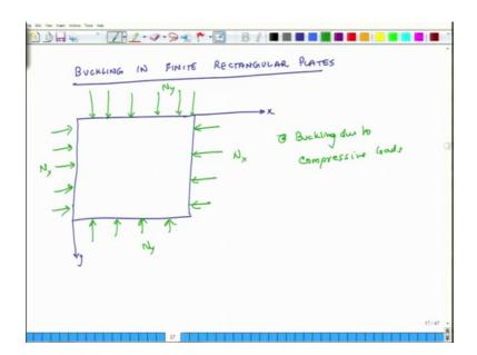
So, suppose so this we will we will discuss about buckling in finite rectangular plates. So, suppose there we have a plate of some dimension. Now, this plate, suppose this is my x-axis, this is y-axis, and the z-axis is perpendicular plane of the screen. This plate can buckle, because of three different sets of forces or force resultants.
