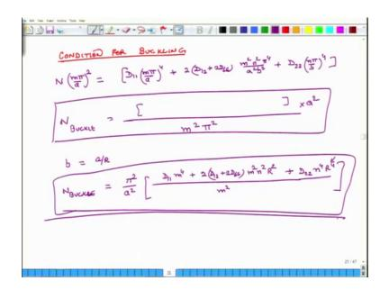
When N equals this right hand side n times m pi divided by a whole square it equals the right hand side, then the condition for buckling have arrived. So, N so N buckle will be what it will be this entire thing divided by m square pi square into a square.
