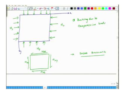
But, the plate can also buckle, if I apply shear loads on it. So, suppose I apply N x y, then also it can buckle. This is called shear buckling, this is called shear buckling. So, the plate will exhibit some shear strain in plane shear strain up to a certain point, but if the external shear stresses shear force resultant N x y exceeds a certain threshold it can buckle, so that is called shear buckling.
