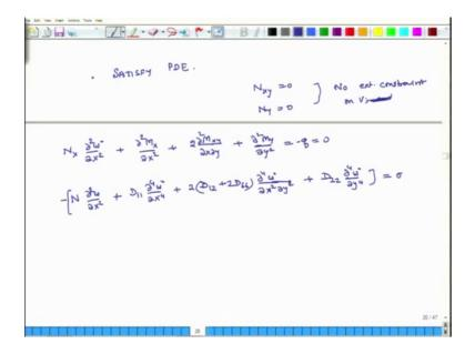
So, if that is the case, then the third thing is satisfy the PDE partial differential equation. So, what is the partial differential equation. So, partial differential equation is N x del 2 w naught over del x square N x y and N y are 0 they are 0, because no external constraint on v and right.
