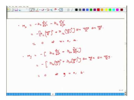
The next thing is M x and M y, M x should be 0 on x is equal to a, and x is equal to 0, and M y should be 0 on y is equal to 0 and y is equal to a. So, what is the definition for M x. So, before we create expressions for M x I should state very clearly that this plate is symmetric an orthotropic ok. It is symmetric as well as orthotropic.
