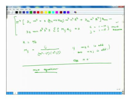
And what we will do is we will see how to use this particular equation and calculate the value of shear buckling ok.
