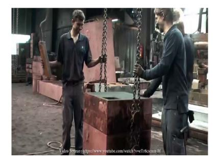
Now, the halves of the mold are parted to remove a pattern.
