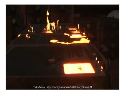
While cooling down, the iron and the other components, mostly carbon, will form microscopic crystals. And, their shape influences the material properties; this will be ordinary cast iron with lamellar graphite also known as grey iron.
