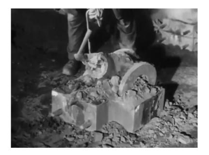
The molder also controls the pouring of the metal. Later he breaks down the mold, the core sand is broken out from inside the hollow casting, which is then fettled and machined.
