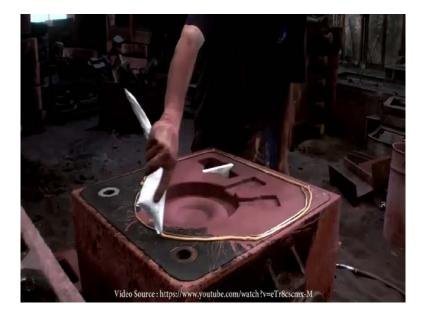
Now, the filter is inserted, and some fireproof putty is laid around the cavities in the mold.
