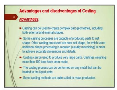
In case of casting, some casting processes are capable of producing parts to net shape. Other casting processes are near net shape type for which some additional shape processing will be required. Usually, they are machining in order to achieve accurate dimensions and details, this we said last time.
