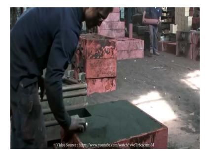
The iron will fill this space and provide additional liquid iron when the molten iron in the wheel is cooling down and shrinking.
