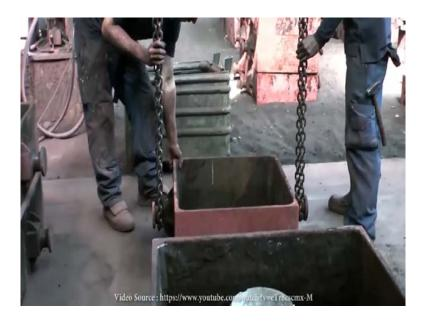
First part of the process is of the preparation of the mold. The bottom half of the molding box or flask is set onto the floor, where one part of the pattern is laying.
