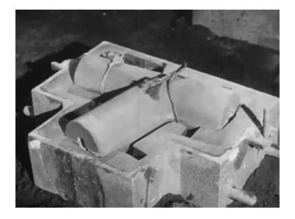
For a hollow casting a core of baked sand is used to prevent the molten metal from filling the whole space left by the pattern in the mold.
