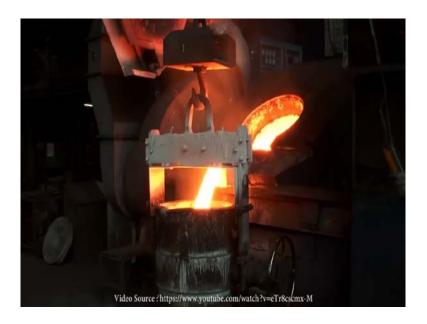
When the temperature is above 1350 degrees Celsius, the iron is filled into a casting ladle and brought to the molds.
