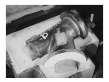
Dry parting sand on the mold face ensures clean separation of the two halves of the mold later.
