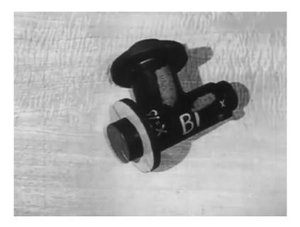
How are such castings made? From the original machine drawing of the required part a wooden pattern is developed.
