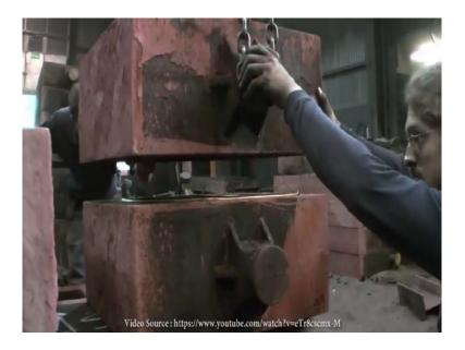
Now the top is set upon the bottom and the two parts are pressed together with clamps.
