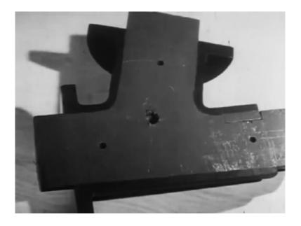
Dowels in one part and sockets in the other, ensure perfect registration when the two pieces are put together.
