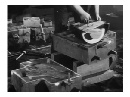
The two mold boxes are kept in correct alignment by register pins. After separation, the patterns are withdrawn from the two half molds, the bottom half of the mold is called the drag, the top half the cope.
