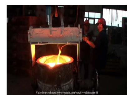
The final measurement of the temperature, when about 80 kilograms of cast iron are poured into the mold.
