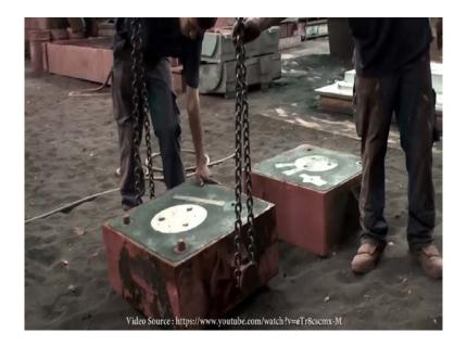
The two protruding knobs that are visible on the top part are there to interlock the two parts in the right position.
