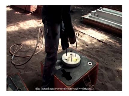
So, that is the moment when my threaded inserts in the model become important. Three hooks are screwed into them and with carefully knocking upwards, the pattern will eventually come loose. Of course, the pattern has to have no undercuts and the vertical surfaces need to be slightly tapered.
