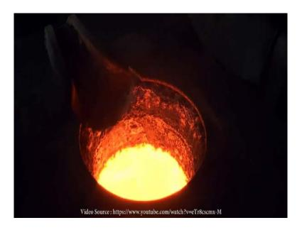
The second part is of the casting process itself. Here is the liquid iron in an induction furnace, slag is removed from time to time.
