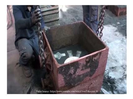
It is now in the same position as it will be later for pouring. After cleaning away the dust the top molding box the cope is set upon of the bottom one the drag.
