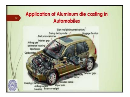
Application of aluminum die casting in the automobiles is shown here and you can see the different parts are labeled here in this diagram. You can see that many of these parts are made by the casting.
