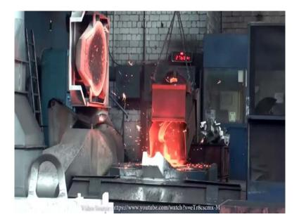
But the furnace is not full yet. So, another container of scrap metal goes into it; maximum load is 3.5 tons.
