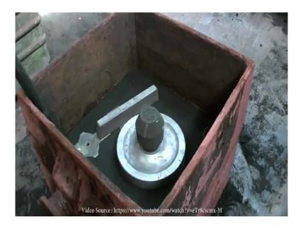
Then, the other half of the pattern is put in place, also the other parts of the sprue pattern and an internal feeder.
