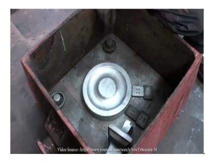
The oddly shaped block in the corner will form a cavity to hold a special filter to keep the slag out. The other blocks are sprue patterns, they form the channels, which will lead the molten iron to the mold cavity.
