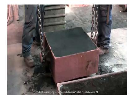
The flask is filled to the rim and after some compacting the top is trimmed flush with the rim. After 10 to 15 minutes the resin that is mixed with the sand has hardened. So, the mold can be turned upside down. (Refer Slide Time: 21:15)
