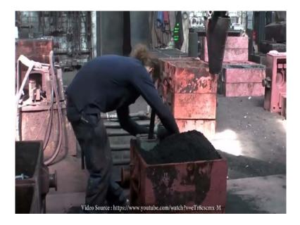
The internal feeder is covered with sand completely. It is just the cavity with an opening towards the pattern.
