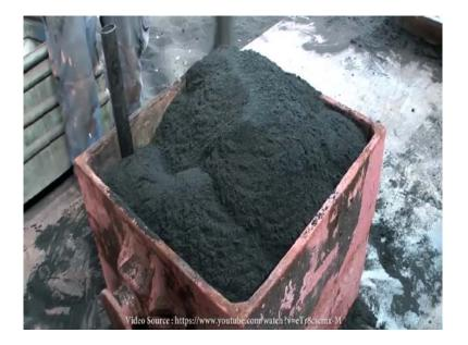
The graphite powder is used to make it easier to separate the patterns from the mold later; on the left an iron pipe is visible, that is the pattern for the vertical parts of the sprue. (Refer Slide Time: 22:48)
