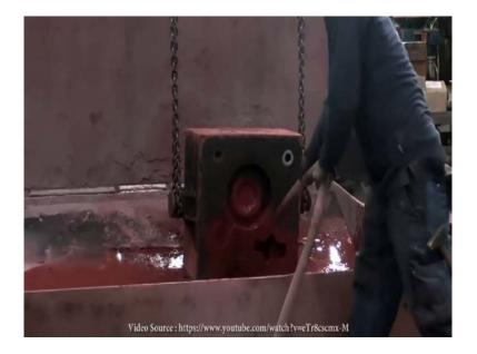
Next step is the preparation of the mold for the casting. This reddish liquid is a suspension of shamud, it will form a thin layer on the mold as a protection against the heat of the liquid metal.
