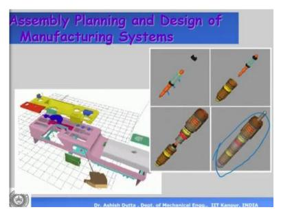
Assembly, so in assembly when you are putting different parts together you are assembling different parts. So, there has to be some sequence and that sequence is basically what we call by assembly planning. So, when you are assembling a product like this, they will have some particular sequence first the red part goes then the black then the maroon part in the roller. So, that order is also a plan and it is basically a motion plan because these things are being moved and assembled together.
