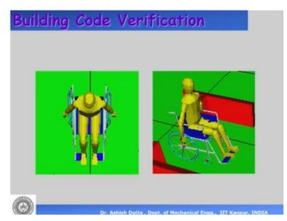
Building code verification is very important these days in which after a building is to be are made the building should be accessible to people using wheelchairs for example. So, before you actually do the construction of the building, they have to check it in virtual reality that wheelchairs can be moved in all places.
