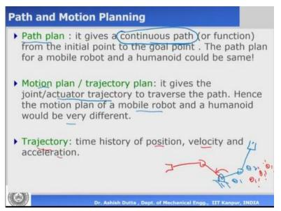
What are the definitions of a path and a motion plan? So, path plan is essentially it gives a continuous path. It has to be continuous from initial point to goal point. The path plan for a mobile robot and a humanoid robot could be the same as I said that a mobile robot and a biped robot could have the same path but their motion plan could be different. So, it gives a continuous path or function so it has to be continuous it cannot be discontinuous.
