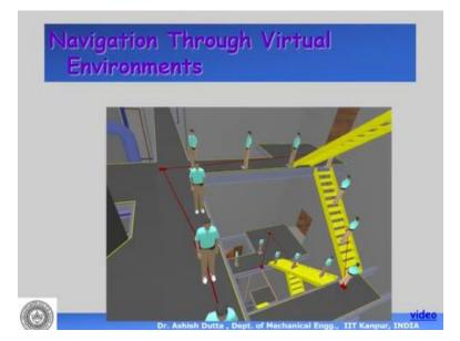
Navigation through virtual environments, so before building a building before actually constructing a building they would actually make this kind of virtual walk throughs to see whether human beings can walk everywhere, if there is a problem of falling down somewhere every place is accessible or there are some places which are not accessible. So, this is basically which is called virtual environments or virtual walk through.
