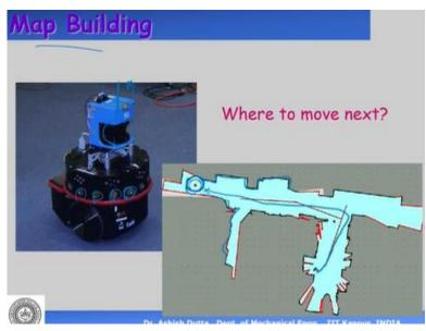
This is the case of map building for example exploration a mobile robot like this which has ultrasonic sensors in front. So, these ultrasonic sensors which can sense the distance and this is a ladder so it is a line laser. So, when it is going along it can it can this can rotate about this axis by 360 degrees. So, when it is traversing it can see, where are the walls and as it is moving it can build its map. So, for example map building inside a building.
