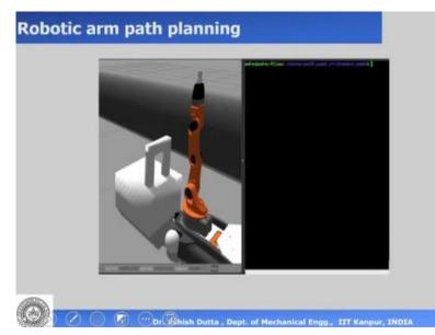
This is the example of robotic arm path planning. So, this is a robotic arm it has to go and go inside their let us say the robotic arm has to go and position itself such that the gripper is inside there. So, what are the different parts that it can follow it has to follow? So, obviously there will be many paths and then once it has done got the path there should be a motion plan which will actuate the joints.
