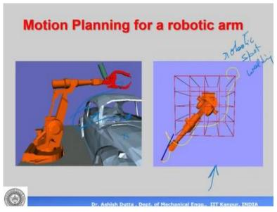
Next motion planning for robotic arm: For example, in automobile industries all these spot welding that are done on cars on the automobiles cars trucks all this. This spot welding is done by robots. So, this robot has to go inside the car and do spot welding, for example if there is a weld here then the robot will have to go like this like this go inside and then do the weld. So, this is not a very simple kind of space where we can say that this is my free space and that is occupied space.
