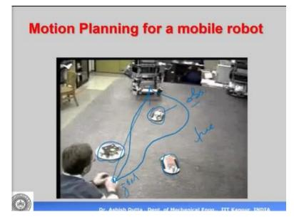
At the simplest level it is a mobile robot maybe can be one mobile robot can be two mobile robots it has to go from maybe these are obstacles. It has to avoid this obstacle, there is a mobile robot has to avoid all these obstacles and go like this and come here. So, motion planning of a mobile robot avoiding obstacles. This is flat ground so this is my free space, this is obstacle space so it is not a very difficult problem.
