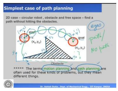
Now the simplest case is this one the simplest case of path planning. Now this figure shows you an obstacle which is shown like a triangle which is shown here so there is an obstacle and there is a circular mobile robot. Now the circular mobile robot can have two wheels on the sides like this let us say it has two wheels and there is a caster wheel in front this is a differential drive robot. Now this robot is required to go from the start point to the goal point that is the task.
