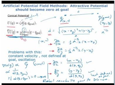
So, what we saw in the last class is that the attractive potential can be a conical potential which is equal to U which is,  $U(q) = \zeta d(q, q_{goal})$ . So, as shown here if  $q_{(x, y)}$  is present position of the robot, and  $(x_g, y_g)$  is the goal position of the robot, then d is the distance between the goal and the present position of the robot and if you write this as d, then the distance is given by  $d = \sqrt{(x - x_g)^2 + (y - y_g)^2}$ .
