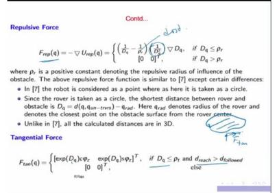
For the repulsive I can have exactly the same. So, this is the repulsive gradient  $F_{rep}(q) = -\nabla U_{rep}\left(q\right) = \left\{\left(\frac{1}{D_q} - \frac{1}{\rho_r}\right)\left(\frac{1}{D_q^2}\right)\nabla D_q \text{ so, it is exactly the same what we are using in}\right\}$
