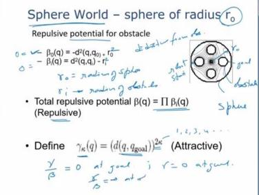
So, once that is function is this one which we call the sphere world, now in the sphere world, you can imagine this to be a sphere. So, this is a sphere that is a spherical and these are obstacles, these also spherical like ball. Now, this is my goal point and it is the robot start
