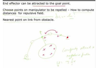
So, this is how we basically do path planning for serial manipulators.
