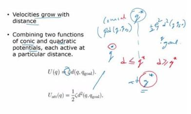
So, what we can do is that we can use both of them the conical and the quadratic potential functions using each of them at a particular distance. For example, we define a distance q \* and when the robot is at let us say at point q and the distance is d which is the distance between the goal and the person position  $d \le q$  \* then we say we have to use the conical function and when the robot is d > q \*.
