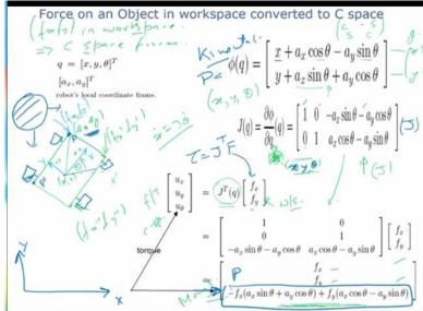
Now, what is the use of this? the use of this essentially we can use this principle when there are multiple forces acting an object. Let us say this is a mobile robot, it has 4 wheels and this is my global frame x axis, y axis and with respect to this, the coordinate of this point is (a  $_x$ , $a_y$ ). And the local frame is here x'y'. So, now what I can say is that suppose there is an obstacle here, this obstacle is applying a force f  $_x$ , f  $_y$  at this point so let us call this point P.
