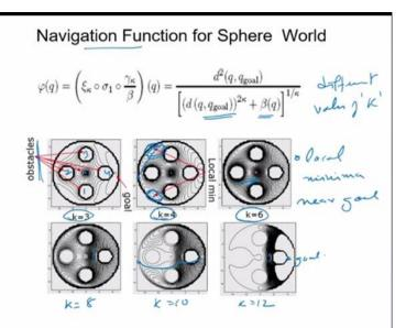
So, if I can define a function like this now we are defining the function this way our cost function maybe, which is  $\varphi(q) = \left(\xi_k \sigma_1 \frac{\gamma_k}{\beta}\right) (q) = \frac{d^2(q, q_{goal})}{\left[\left(d(q, q_{goal})\right)^{2k} + \beta(q)\right]^{\frac{1}{k}}}$ . So, I am defining
