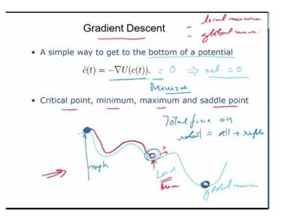
So, now let us look at how to use the gradient descent method. So, we take the potential, the effective force acting on the robot, so total force on robot is equal to repulse attractive plus repulsive force. So, I use the gradient descent that means I do minimize, so it is a minimization problem. So, basically, what it means is that minimizing the potential energy. So, you can imagine if there is a ball that it has a potential energy mgh when the ball comes down, this decreases.
