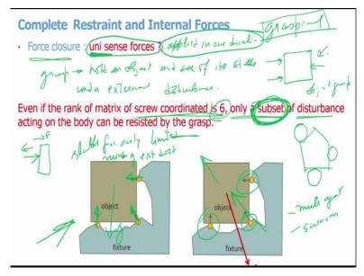
Now first let us look at the grasping. Now this is an object which is being grasped for an object here which is shown in the figure, this is an object and it has 3 contacts which are there; one contact here, one contact here and one contact here. Now we can assume this to be something like a box which is caught with two fingers, three fingers like this, the same thing or let us look at an object with multiple mobile robots.
