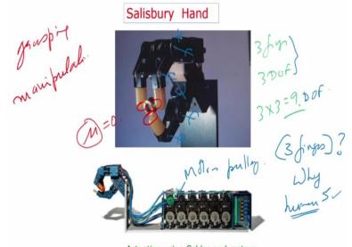
Actuation using Cables and motors
