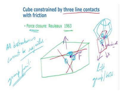
And for example, this is the example he also gave. So, this was invented first way Reuleaux in 1963 very long time ago. If you take a cube, this is a cube and we are holding it by three line contacts. So, a cube constrained by three line contacts with friction. So one line is like this, one line is like this and one line is like this. I can also give the idea that if this is a cube, let us say it is a cube, I am sure you must have felt this or seen this or experienced this somewhere.
