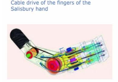
This is showing the internal construction of the finger motion. So, there are cables. These cables are going through the pulleys and then are connected to particular joints, like this is connected here. This one is connected through the cable is connected here. So, when this cable tension changes, what will happen? This joint will move that is how the fingers of a multifinger hand moves.
