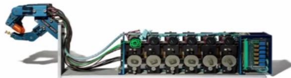
Actuation using Cables and motors
