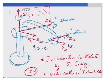
So if you can visualize, there is a link is like this and there is a link here. That is a link and this can rotate about this, so that is my base. And if you can imagine, then this is my axis that is the first axis so this can rotate like this, that is the second axis which can rotate like this. And there is a third axis which can rotate like this. These are axis 1, axis 2, axis 3. I hope we can imagine. So this is something similar to our waist.
