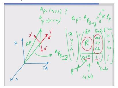
Then we moved on to the homogenous transformation matrix and we said that if you have a frame, this is my fixed frame. Let us call it frame A and this is x, y, z. Now, if you have another frame which is rotated and translated with reference to this, so I have another frame which is rotated and translated. So this is my frame B, and this is my x', y' and z'. And suppose I have the coordinates of a point in frame B.
