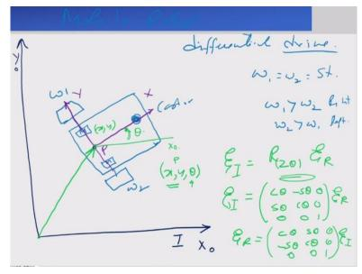
Now, let us move on to a mobile robot. Let us say in the case of mobile robot, what is the relationship? So mobile robot. So in this course, we will be dealing with mobile robots and also will be dealing with serial arms. So, this is a mobile robot, a differential drive mobile robot which means that there are two wheels which has  $\omega_1$  velocity and this one has another velocity  $\omega_2$  and there is a castor wheel there, which basically supports differential drive with castor wheels.
