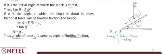
Along with the concept of friction, we need to understand something known as Angle of Repose. If there is a body that is sliding over a slant surface with a slant angle of  $\theta$  and the normal force acting on the body from the bottom is N. Frictional force that is acting on the body F is determined here.
