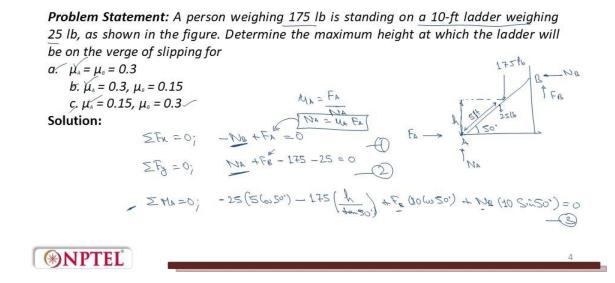
Let us now try to see some examples on Friction and Moment of Inertia. So, here is one problem statement where a person weighing 175 pound is standing on a 10 feet ladder weighing 25 pound as shown in figure. I will draw a figure here. This is a ladder that is 10 feet long and a person is standing here who is weighing 175 pound. Determine the maximum height at which ladder would be on verge or slipping for.
