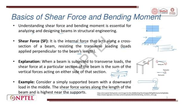
Basics of Shear Force and Bending Moment. Understanding shear force and bending moment is essential for analyzing and designing beams in structural engineering.
