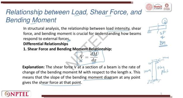
What is the relationship between Load, Shear Force and the Bending Moment? This is what comes to your mind. I have a structure or I have a flat plate or I have a scale. Now in this scale, I try to apply load. So now I try to fix this point and I try to apply load. So now I
