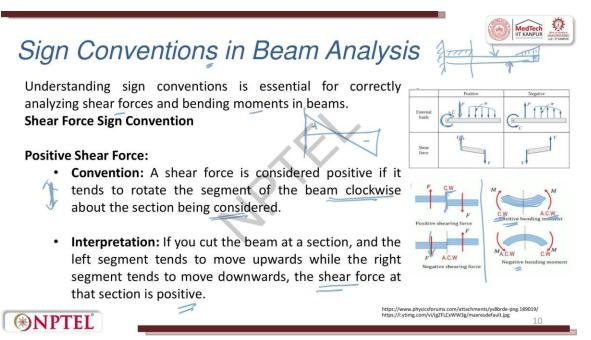
The next important topic for discussion is going to be the sign conversion in beam analysis. It is very essential for you to understand correctly what are the signs which are used while analyzing the shear force and the bending moment. As I told you, when you try to have a shear force like this thing. So, if you take positive, negative. So, how did this come positive and why is it considered as positive? Why is it considered as negative?
