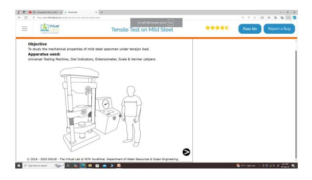
In the simulation, you see, it has been shown that this is the objective, to study the mechanical properties of mild steel specimen under tension load.
