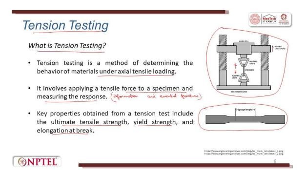
So, what is a Tension Testing or Tensile testing? Tension testing is a method of determining the behavior of material under axial tensile loading. So, material is under a load, we are pulling apart the material in two different directions, a specific setup.
