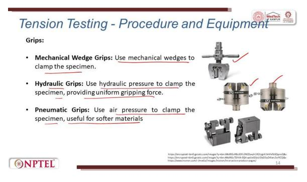
Let me also show you different grips. These are different grips that I just mentioned in the previous slides. You can see a mechanical wedge grip use mechanical wedges to clamp the specimen, there are mechanical wedge grips using just a mechanical force itself.
