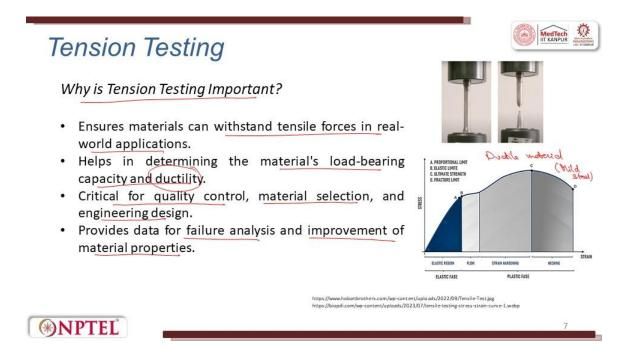
Now, what is the importance of tensile testing? Why is Tension Testing Important? It ensures materials can withstand tensile forces in real-world applications. It helps in determining the material's load-bearing capacity and ductility.
