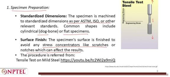
First and the foremost point is the first step here is preparation of the specimen. So this is a typical specimen. The specimen is elongated here. The force is on both the directions here and it is getting elongated. Standardized Dimensions. The specimen is machined to standardize dimensions as per ASTM, ISO or other relevant standards. Common shape include a cylindrical dog bone or flat specimen.
