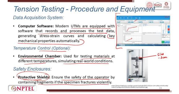
And there are computer software available in modern Universal Testing Machines are equipped with the software that records and processes this test data generating stress in curves and calculating key mechanical properties automatically.
