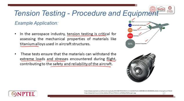
Now comes the Application. You can see in aircraft, different materials are there. 10% of that is steel, 15% is titanium. Titanium you know is having high strength to weight ratio with a very low weight strength is very high because weight is a major consideration when we are trying to design an aircraft. So titanium is there, aluminium is there. And advanced composites are there nowadays, 50 percent of the material is advanced components, 5 percent of the materials are also there.
