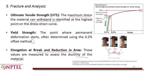
Then we try to conduct the Fracture and Analysis that is Ultimate Tensile Stress. The maximum stress the material can withstand is defined as the highest point on the stress strain curve. So, this is ultimate tensile strength that is shown here. Yield strength is the point where permanent deformation starts often determined using 0.2 percent offset method. So, here is the yield strength.
