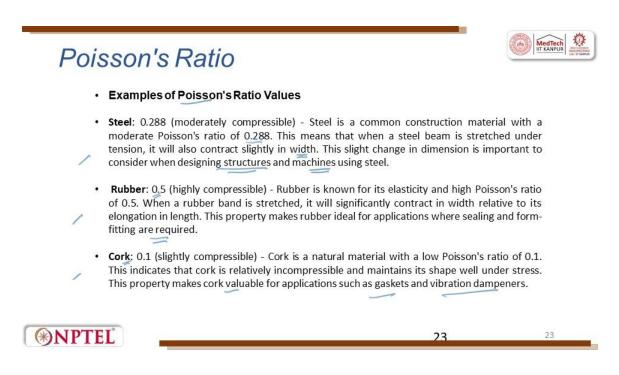
So, examples of Poisson's ratio values, steel it is 0.228, Steel is used commonly for construction material with a moderate Poisson's ratio of 0.8. This means that the steel beam
