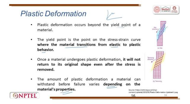
The plastic deformation generally occurs beyond a yield point. This yield point is a point on the stress-strain curve where the material transitions from elastic to plastic behavior. So, from elastic to plastic, once a material undergoes plastic deformation, it will not return to its original shape even after the stress is removed. So here if you see that there is a slip which is happening and there is a twin direction which is there.
