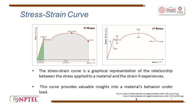
So, this is the Stress-Strain graph for a typical material. So, you have a stress in the y-axis and strain in the x-axis. We have already seen the elastic deformation which is the elastic limit. After the elastic limit starts the plastic. So plastic limit. So elastic limit point and then you have a fall down, fall up. Then you see a yield started increasing. So, this is a yield point.
