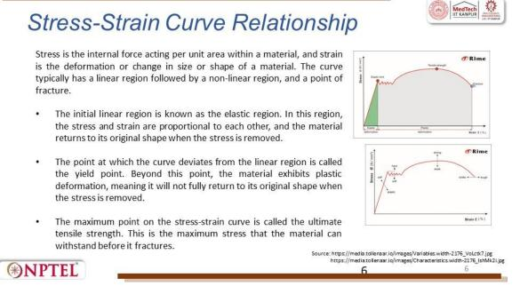
So, the stress is the internal force acting per unit area within a material. Strain is the deformation or change in size or shape of the material. The curve typically has linear region followed by a non-linear region and a point of fracture. The linear region is known as elastic region. In this region, the stress-strain are proportional to each other and the material returns to its original shape when the stress is removed.
