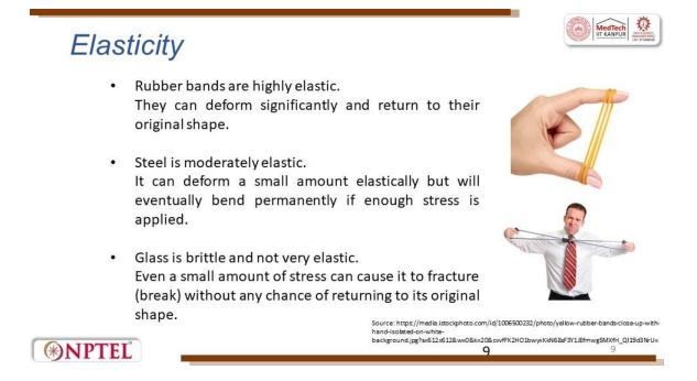
Rubber band are highly elastic, they can deform significantly and return to its original shape. Steel is moderately elastic. It can deform a small amount elastically but will eventually bend permanently if enough stress is applied.
