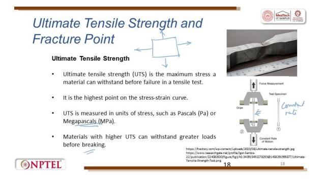
Ultimate Tensile Strength (UTS) is the maximum stress a material can withstand before failure in a tensile test. It is the highest point on the stress-strain curve. It is always reported for a typical metal in Mega Pascal (MPa). Materials with higher UTM can withstand greater loads before failure. After you cross the ultimate tensile strength point, you move towards the failure.
