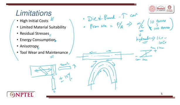
Saying this, it also has some disadvantages because it is used for higher production, repeatable, reliable processes. The initial cost is very high. That means the die and punch costs are high. The second thing is, if I have to apply huge pressure, what is pressure? Pressure is nothing, as I told you—it is force per unit area. I need a machine which is used for doing it.
