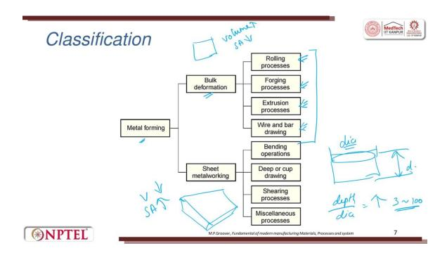
Now, let us see the classification of metal forming process. The metal forming process is classified based upon the raw material available. If the raw material is in an ingot form where the volume is high and surface area is low. They fall under the category called bulk.
