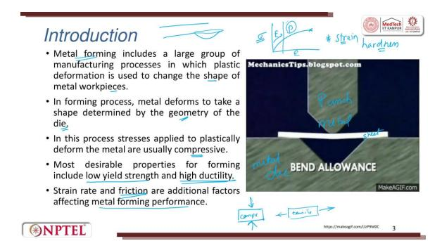
So, metal forming includes a large group of manufacturing processes in which plastic deformation is used to change the shape of the metal workpiece. When you look at the stress-strain diagram, We had for aluminum alloys; we had for aluminum alloys like this. So, you will have the elastic limit, then you will have the plastic region. So, when we are doing metal forming, we cross the elastic state, enter the plastic region, and then try to shape it.
