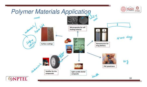
Here are some of the major applications of polymer materials. They can be used for making microcapsules for self-healing materials. Self-healing materials mean you take a material, puncture it, or crack it. When these self-healing capsules are applied, these cracks are arrested and closed. These are microcapsules made out of polymers that have self-healing properties. You can also create surface coatings out of polymers.
