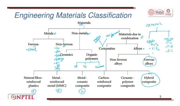
Materials can be classified in many ways. The most basic and fundamental way is that they are classified into three parts. One is Metals, Non-Metals, and Materials due to combination. You are trying to combine materials. Materials here may be between A and B of Metal and Non-metal to get an output. So, they are classified into three basic steps: Metals, Non-Metals, and Materials due to combination. It might look a little surprising.
