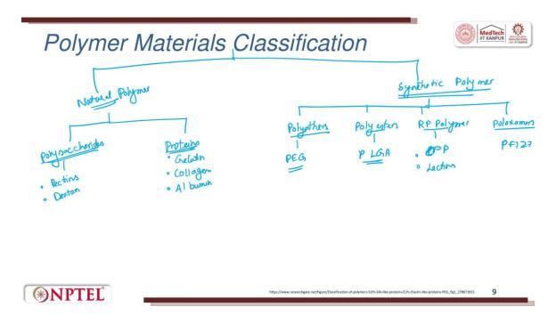
So, Polymer Material Classification. So here, polymer is again classified into two types. One is natural polymer. The other one is synthetic polymer. Synthetic polymer means it is artificially made.
