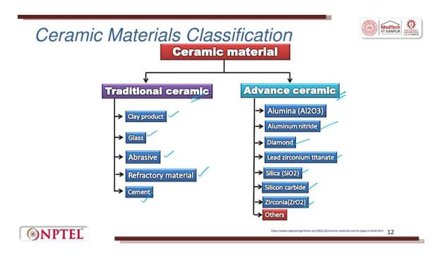
Ceramics are also classified into two types, which are called traditional ceramic and advanced ceramic. Earlier, I classified them into oxide and non-oxide, but here we are classifying them in a different fashion, which is called traditional ceramic and advanced
