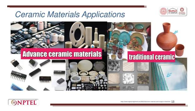
So, here are some of the examples where you see a lot of applications. If you see an IC chip, a silicon wafer, it is all ceramic material. You can see, these are all alumina, Al2O3. These are some of the things which are used for engineering applications. In ball milling operations for grinding powders, we use zirconium oxide balls. When you want to hammer and break, we try to have these balls.
