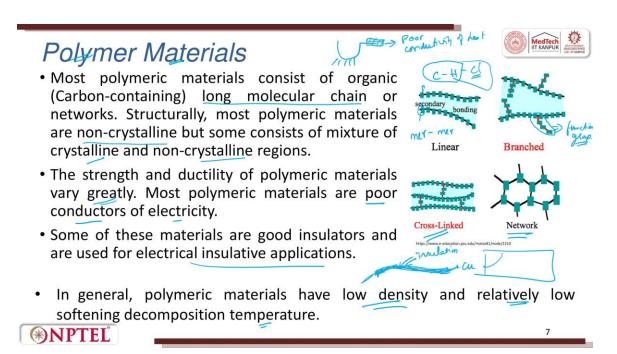
When we look into polymers, polymers are made out of C and H, carbon atom, hydrogen atom and then you can try to have some other atom to bring to the or add value such that you get a good engineering application. Most of the polymer material consists of organic carbon content. These carbon content are all formed into a chain.
