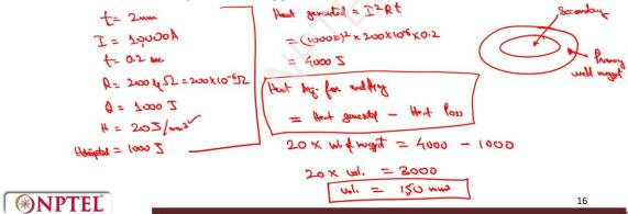
Let me come to the problem statement. Two sheets of 2 mm thickness are spot welded by supplying a welding current of 10,000 amps for 0.2 sec, and contact resistance is 200  $\mu\Omega$ . Heat dissipated to the base metal is 1000 J. Heat required for melting is 20 J/mm³. What is the volume of the weld nugget?
