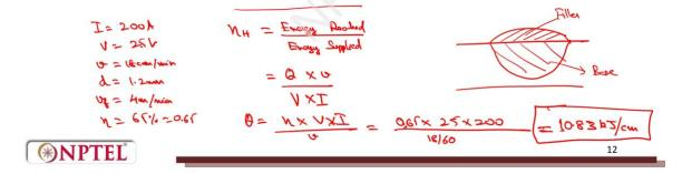
Here, we are using an inert metal gas welding process with the following parameters:
