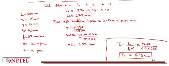
A hollow workpiece of 250 mm long and 40 mm diameter is to be turned in 4 passes. Calculate the machining time if the approach length = 15 mm, over travel = 10 mm, feed = 0.7 mm/rev and cutting speed = 32 m/min.
