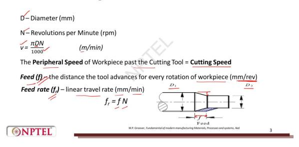
Now, if we are given the diameter and the RPM (rotational speed), we can calculate the cutting speed or the peripheral speed using  $v = \frac{\pi DN}{1000}$ . The factor of 1000 comes into play because we are converting the diameter into meters, as meters per minute is squared, and the diameter is generally given in millimeters.
