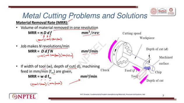
Then, we sometimes have to calculate the material removal rate. Material removal rate is in three forms. That is, material removed in one revolution, Then, N rev/min, then depending upon the width of the tool and the depth of cut, this is also calculated.
