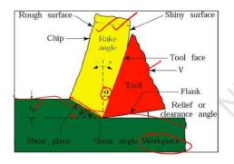
α : Rake angle β : Frictional angle F: Frictional Force
