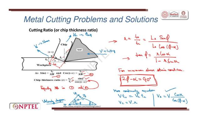
Here, you can also see it is again given the rake angle and the shear angle. We have the length of the shear plane here. This is my Ls, the length of the shear plane. Here,
