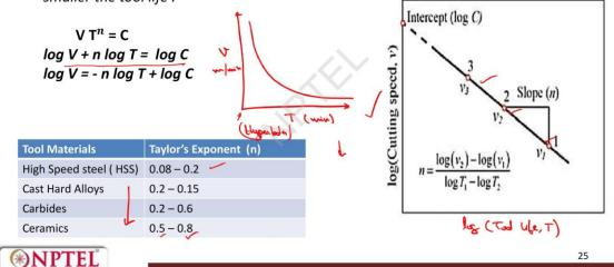
So here, tool life is mainly affected by cutting speed, meaning high cutting speed, smaller the tool life, as it is given here. If we take log on both sides, log  $V + n \log T = \log C$ . This is generally calculated. This becomes a simple equation of a linear line.
