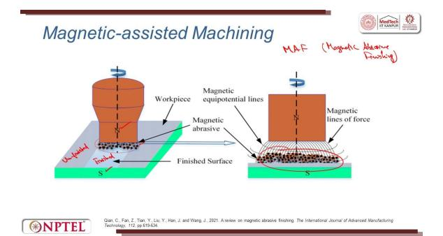
Next is magnetic assisted machining. When you use machining using magnetic assistance, the tool is magnetized specifically in reamers. The cutting edge is having longer tool life.
