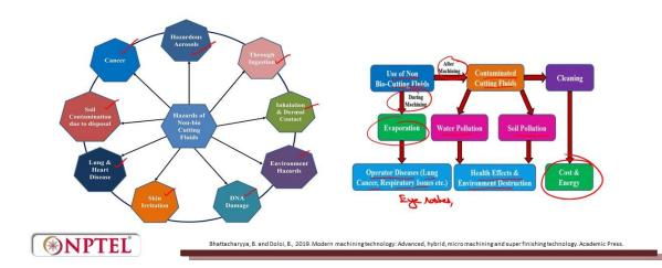
If bio-based cutting fluids are not used, there are certain hazards associated with non-bio-cutting fluids, such as synthetic cutting fluids. The hazards of non-bio-cutting fluids include hazardous aerosols, which are generated, as I just mentioned.
