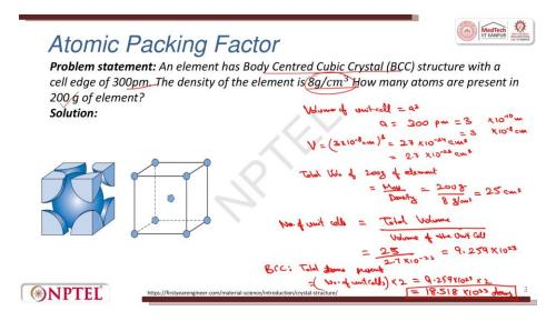
Let me directly come to the problem statement and let us try to solve it. The statement says an element has a body-centered cubic crystal, that is BCC, with a cell edge of 300 p.m. The density of the element is 8 grams per centimeter cube. How many atoms are present in 200 grams of the element? It is so simple here.
