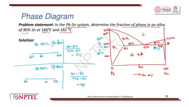
I will give one problem of another phase diagram. Let me see, this is a lead-tin system where they are asking to determine the fraction of phase in an alloy of 80% tin at 184 degrees centigrade and 182 degrees centigrade. In lead-tin, what happens? So, I have lead on the left side and tin on the right side.
