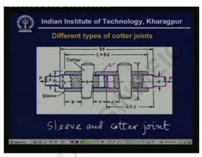
now this was the very simple joint which is known as as a sleeve type cotter joint so this is known as sleeve and cotter joint
