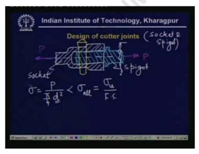
first of all let me draw a cotter joint here we are going to use the socket and spigot type joint now this spigot this is a socket it has hole inside and we have another component which is known as spigot this part is spigot and through it we insert what is known as a cotter so this is the cotter inserted
