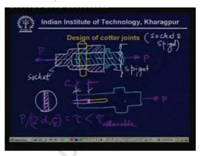
again this is this the spigot and this is the cotter [Vocalized-Noise] now if the force is given here then a large force is developed large stress is developed and that stress may be such that this part gets torn away it is it may fail against this direction
