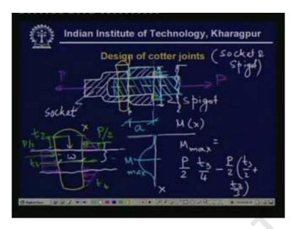
the bending moment diagram is so this is m x x over here so the bending moment diagram is almost look like that of course not zero over here
