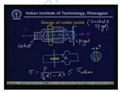
and the cotter is inserted over here this is the cotter insertion point so therefore and this uh this a circular cross sections so therefore the critical cross section will be somewhere here and if you find out the if you draw the cross section then it looks like here through which the cotter pass the cotter passes so this is the critical cross section of the spigot
