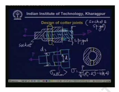
if we draw the socket part so this is the socket and we have a cotter [Vocalized-Noise] passing through here
