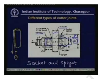
now [Vocalized-Noise] what you see here is one kind of cotter joint and here you see this part there are two parts which are to be joined by means of a cotter
