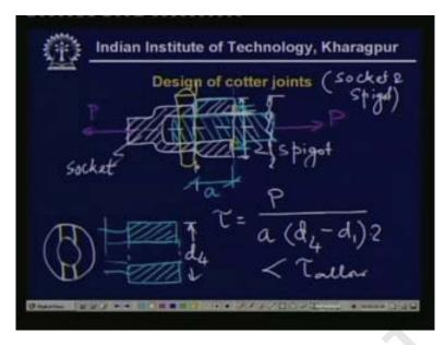
this is the spigot collar and this entire surface so this part is subjected to the shear shear stress and the shear stress is nothing but tow will be equal to P divided by this total area which is equal to this distance a times this part that is if you draw the cross section it becomes so this length this four lengths together times this distance a and that is equal to a times the outer diameter which is let us say we take this to be d four
