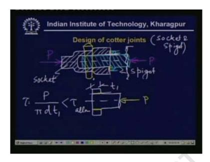
now this is the collar and the shear takes place over here if the force is too large we have P over here so the shear occurs over here so what is the total surface now this is cylindrical so therefore the total surface area is nothing but pie d and this diameter which is equal to which is equal to d pie d times this thickness t one
