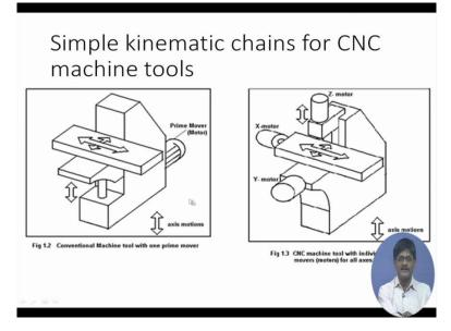
For example, you would see a milling machine in which we have 3 motions X, Y and Z and there is a motor which is also providing the cutting speed. Instead of this, on the CNC
