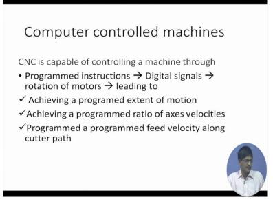
In computer-controlled machines, instead of devices like cam, et cetera, there are programmed instructions which go inside the machine and I mean when they are executed the program instructions, they develop digital signals which might be ultimately rotating motors at a definite rate and this leads to achieving a definite extent of motion and achieving a particular ratio of the of the axes velocities okay. And also it results in attainment of programmed feed velocity along a cutter path.
