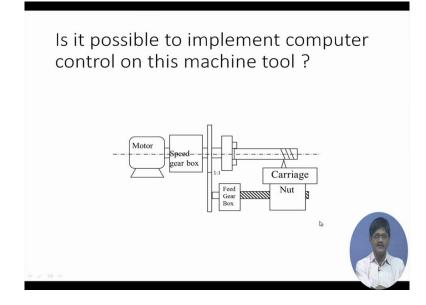
So in this machine is we want to implement computer control, we can see that there is a chain moving from the top up to the spindle and there is also power flowing this way so that the same motor through gearboxes is controlling 2 motions, this has to be removed and a separate motor has to be put for the feed motion, so one motor for the feed motion, one motor for the speed motion and yet another motor would be required for a cross feed, one for Cross field, one for longitudinally feed okay.
