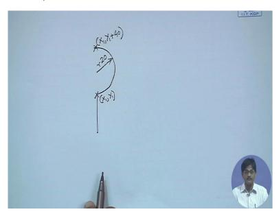
Suppose you are heading this particular body, from here I go up to this position and then I take a turn and come to this particular location. So if I know the radius of the circle like R 20 it is very, it is extremely simple for me to calculate this particular coordinate location, I will say this is X 1 and this is Y 1. If these are known to me, then I can definitely say this point
