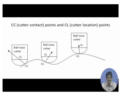
First of all, we are differentiating between 2 types of points in connection with 3 axis machining that is, if we have a ball ended milling cutter in connection with the surface, the point at which it connects to the surface the point of touch or contact, it is called cutter contact point CC point. So this is one cutter contact point, this is another cutter contact point
