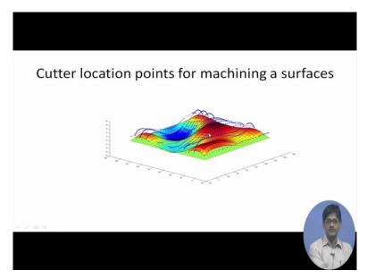
Here we have shown a surface and you can see some small red or rather blue dotted lines just over that particular surface, these are cutter paths that mean the centre point of a ball ended cutter path with these locus point as the centre points of the ball end okay, we will have an example later also in order to understand this.
