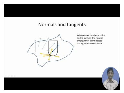
So this is the cutter, when the cutter is touching the surface at this point the normal to the surface will essentially contain the centre of the cutter okay. So the normal to the surface will essentially contain the centre of this spherical end of the cutter, so we understand that this normal which is emanating out at this point of the surface it is passing through this centre which is shown, so we make use of this... This figure will make it clear.
