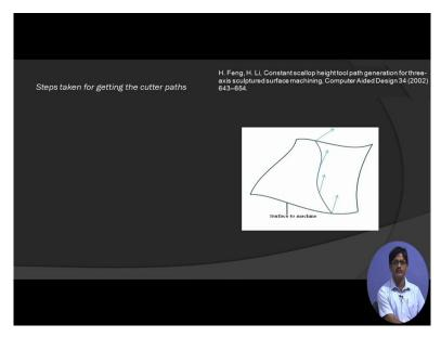
So this cutter path to start with, we mark at particular points which are forward steps adjusted, we determine the surface normals at these points. These points are the CL points, the centers of the nose portion of those ball end milling cutters. We join them by a smooth curve, we find out that tangents to this smooth curve hence we get the cutter directions at these respective locations.
