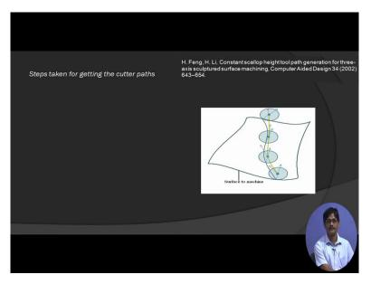
Next we draw the swept section of the cutter end cutter ball end at these respective locations and swept sections are the once which define the geometry of the groove being cut. We remove all the construction lines.
