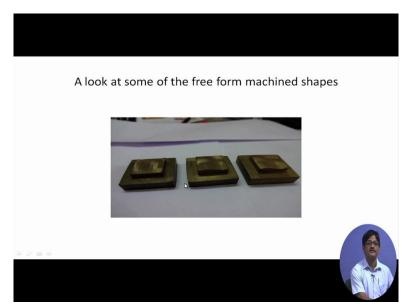
So at the end of this discussion, we come to 3 examples of jobs which have been cut with different forward steps and different side steps. As you can well identify, this one has large forward steps and also a very coarse side step pattern so that roughness will be visible to the naked eye while these are not so a closer look perhaps, yes.
