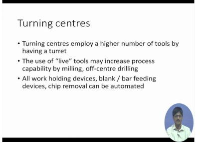
Turning centers also employ a higher number of tools by having a turret and if "live" tools can be used that means tools which have their own motors for making them rotate, then milling, off-centre drilling, these operations would also be possible. Apart from that, work holding devices, blank or bar feeding devices, chip removal, all these things can be automated, which makes the turning centres much more versatile than ordinary CNC lathes.
