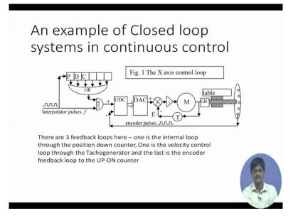
This is an example of closed loop system in continuous control. Continuous control as we have discussed, it is another type of classification in which a system which is capable of moving the table in straight line we nearly that is along a straight line at a predetermined rate and also it is able to coordinate the motions of 2 axis so as to produce circular motion that is these are the examples of continuous control.
