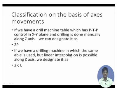
There can also be type of classification depending upon the type of axes movements available, let me give you some examples. If we have a drilling machine table which has point-to-point control in X-Y plane and drilling is done manually along Z axis, we can designate it as 2P. As the name suggests that there are 2 axes which are moving and they are
