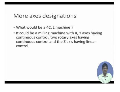
What would be a 4C, L machine? It could be a milling machine with X and Y axes having continuous control, two rotary axes having continuous control and the Z axis having linear control, so X and Y, two rotary axis 4C, L for the Z axis having linear control.
