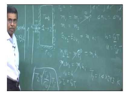
This problem tells that there is a line which connects to a tank which connects to a closed tank this is tank and the tank is insulated it is adiabatic condition there is no heat transfer from the tank, this air is flowing for example in this there is a bulb, now first the valve is open so that the air goes into the tank we take a control volume like this, surrounding the tank and cuts the control surface here where the mass coming in.
