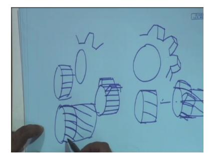
So you have quick look hear I can have the gear of this type you know, the teeth of this type as I have been drawing that means if you look along the axis of the gear the teeth are straight, so that when you draw then you can draw them in this way. But you can also have gears in which that teeth instead of being straight okay, here we are drawn gears which are having straight teeth. That means the teeth are in this way, instead of that they might have this away.
