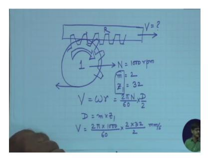
Say I have this has a gear depiction of a gear and this as a rack. Suppose I give this formation this one is root heating, this one is called 1 and this is called R. For R I am interested to find out the velocity it will develop, and here I am having N = 100 rpm, m = 2, number of heat = 32. What will be the speed developed by the rack? So in this case what do we do?
