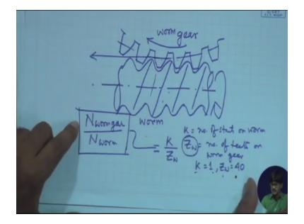
Just now from the first step itself if you can reduce the speed from 400 to 10 by employing k=1, zw=40. As simple as that okay, this is the advantage of the worm and worm gear. This drastic speed reduction in a single stage, there are problem associated to worm gears and sometimes those problems are made use of. For example you know specific helix angles and coefficient of friction, this is self locking.
