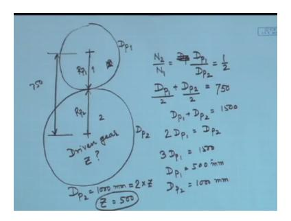
Driven gear each serving the purpose, yes as it is connected with the smaller gear if this has Rpm x this Rpm will be less than x, okay. So because it is larger in size and infact the node here diameter value the exactly the diameter will be brought down by a factor of half, okay. A factor of 2 the Rpm will be brought down by a factor of 2, so everything is satisfied now we have to find out the number of teeth on the driven gear, number of teeth.
