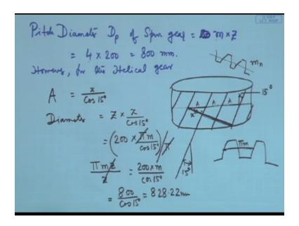
Diameter, sorry pitch diameter  $D_p$  of spar gear = 200 sorry let us give the symbol first, m x z = 4 x 200 = 800 mm. However for the helical gear this is the spar gear say yeah these are the teeth of the helical gear in a helical gear what happens is, that this distance taken normal to the tooth orientation this one corresponds to okay these dimensional if it is sectioned here it will be coming something like this.
