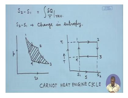
So, we can write S 2 minus S 1 integration is possible. So, it should be dQ by T reversible and S 2 minus S 1 is change in entropy. So, entropy change is related to the process of heat transfer and you see it again heat transfer has got a sign convention. So, accordingly the sign of entropy whether there is a positive change of or increase in entropy or decrease in entropy; entropy being a property that will depend on the sign or direction of heat transfer all right.
