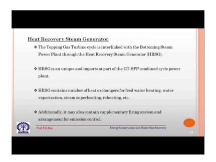
With this I go to a very important device which is part and parcel of a gas turbines steam power plant combination that is, called heat recovery steam generator.
