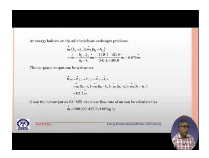
So, first what we like to do the heat exchanger which is there on between the gas turbine cycle and the steam turbine cycle which is also known as HRSG heat recovery steam generator we will do an energy balance for that. Neglecting losses from the HRSG we assume it is perfectly insulated.
