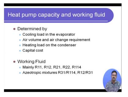
So, with that I will say what is the heat capacity and working fluid. So, what is the capacity going to depend on it is going to depend on what is written in on the slide it is going to depend on the cooling load on the evaporator. So, let us say I am using it for
