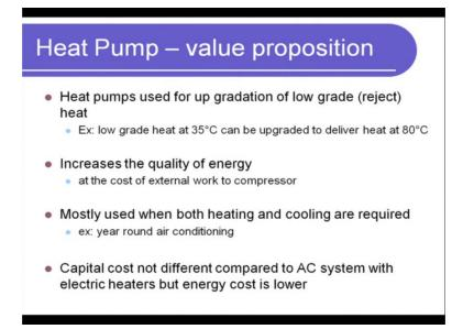
So, let us look at the next slide which is what we are saying here what is the value proposition of a heat pump; the heat pump is used for up gradation of low grade or reject heat. So, let us say low grade heat at 35 degrees can be upgraded to deliver heat at 80 degree centigrade this is 35 and 80 are just 2 numbers that I have picked. So, essentially at a low temperature to higher temperature so that is the value proposition, how do I do this clear and or why do I do this in the first place.
