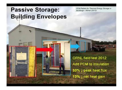
So, this is the motivation. So, what they did was they actually this building material the outer wall they added some PCM to the insulation remember this is here I mean the walls right now over here is not just your brick and brick and concrete, but it will have several layers. So, it has cellulose plus PCM pellets. So, this is some kind of a phase change material that they use.
