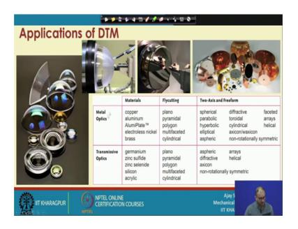
So, if you see oh most of the lenses, most of the lenses are fabricated by the DTM. So, this is one of the application where polymer is being machined on a diamond turning operation, and most of the metals non ferrous mostly because when you are using a diamond as a cutting tool, ferrous materials create problem for because of the carbon migration from the workpiece to the tool and because of that, you will get the different
