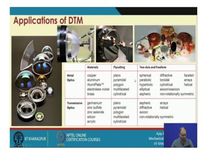
So, these are the different applications of a diamond turning operation of diamond turning machining. So, we can see that it applications there applications are very large in terms of processing of metal components, polymer components and there are many different type of shapes also you can produce by this process.
