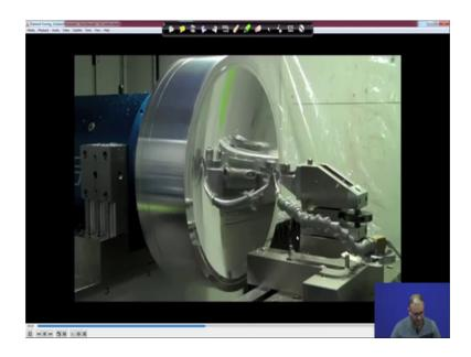
So, this is the one example, now if you see bigger size component now you can say this size is at a meter scale and these particular mirrors are mostly the aluminum mirror, where you want to get some type of a application on telescopic things. And this is the diamond single pole diamond cutting tool and this is the removal of this part.
