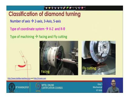
And this is their fly cutting. So, now, how is that these things are different? Now, you can say the cutting tool is located here on a tool pose, but here cutting tool is located on a spindle size or workpiece is on the headstock.
