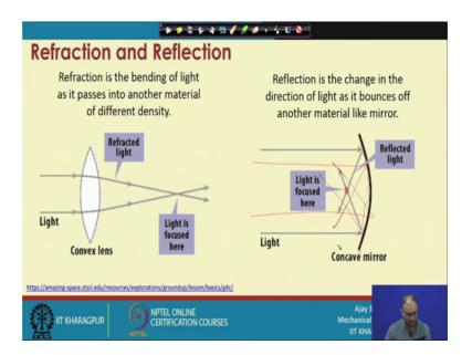
Now, what is the reflection because we can get two different type of things, one is you can fabricate lens also and you can fabricate mirrors also. Now, if you say what is the application of lens that this is there one lens here and live and light is passing through it,
