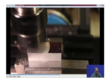
Now, let me show you this is the bigger conventional example, now you can say this is the work piece and this is the cutting tool. So, it is a single point cutting tool, but it attached with the spindle axis of the machine and then it rotates when it rotates it has only single cutting edge, which will remove the material. So, to get this thing down you have to rotate this thing is a high rpm in a very low feed rate. So, you will not get any type of mark on the top surface.
