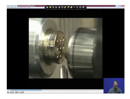
So, it is the tool is now rotating, and you are making a different type of lenses on the surface. So, this is the lens mold.
