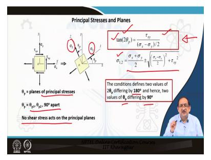
So, following that procedure, we can actually find the angle in terms of tan  $2\theta$  at which the normal stresses can be maximum or minimum so, once we have determined that, we can put the value back in the equation and find out the maximum and minimum normal stresses, which
