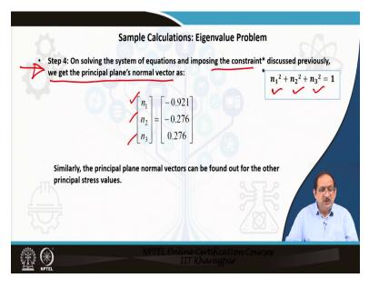
So, in step number 4 we are solving the system of equations imposing the constraint that is the sum of the squares of the direction cosines is equal to 1.
