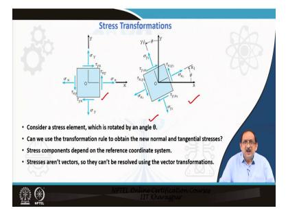
Based on the concept discussed in the earlier lecture, we restate that stress components acting at a point will depend on the orientation of the area on which it acts. So, let us consider a square stress element as shown in the figure on the left, which represents the state of stress acting at a point.
