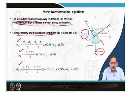
Now, let us find out the equations of the set of stress components corresponding to a new orientation or transformation. Now, the stress transformation is a way to describe the effect of combined loading on a stress element at any orientation. So, from geometry and equilibrium conditions, we can find the equations of the normal stresses  $\sigma_{x1}$ ,  $\sigma_{y1}$  corresponding to the new coordinate system x1, y1 and the shear stress acting on the plane.
