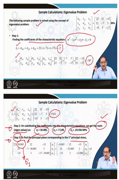
Let us, now undertake some sample calculations on an eigenvalue problem. The following sample problem is solved using the concept of the eigenvalue problem. So, a 3D state of stress is given here. So, the first step is finding the coefficients of the characteristic equation which is stated here.
