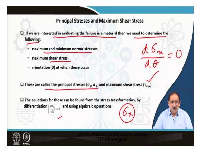
Let us discuss principal stresses and maximum shear stress. If we are interested in evaluating failure in a material, we need to determine the maximum and minimum values of normal stresses
