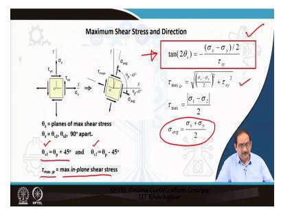
Let us, now find out maximum shear stress and its direction following the similar procedure as done in case of the normal stress, we take a derivative of the shear stress and equate it to 0 to find the condition for which the shear stress can be maximum. So, it comes out to be tan  $2\theta$  equal to an expression consisting of  $\sigma_x \sigma_y$  and  $\tau_{xy}$  and if we substitute this expression in the original equation of the shear stress.
