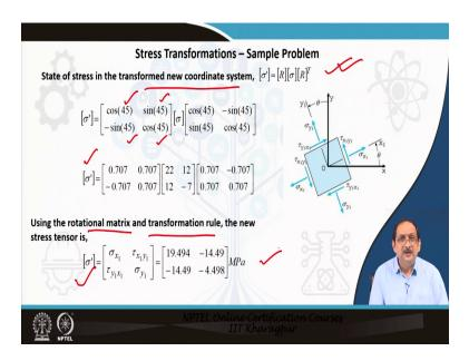
So, we substitute the value of  $\theta$  in this equation and then find out the value of the new stress tensor using the rotational matrix and the transformation rule. So, the new stress tensor is given by  $\sigma$ ' and the values are presented in this slide.
