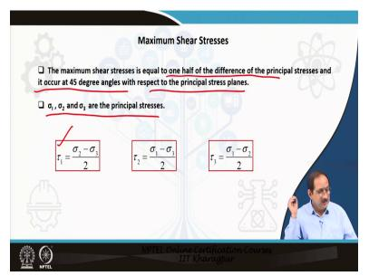
Now, the maximum shear stress is equal to 1 half of the difference of the principal stresses and we have found this out earlier and it occur at 45° angle with respect to the principal stress plane. So,  $\tau_1$ ,  $\tau_2$  and  $\tau_3$  can be determined using the principal stresses as shown here in the slide. So, at  $\sigma_1$  and  $\sigma_2$  and  $\sigma_3$  are the principal stresses.
