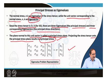
The normal stress  $\sigma$  is an Eigenvalue of the stress tensor while the unit vector corresponding to the normal stress n is the Eigenvector very important the normal stress  $\sigma$  is an eigenvalue and the unit vector or directions corresponding to the normal stress n is an Eigenvector. But, if we consider a 3D problem, then the stress tensor is expressed as 3 by 3 matrix.
