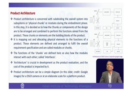
So, what is product architecture? Product architecture is concerned with subdividing the overall system into subsystems or which are called physical chunks, a camera for example, which you can see on the right hand side the block diagram. It is a DSLR camera block diagram. So, closely if you look at later, I am just explaining now because this is not which I would be explaining here, but a in a larger image you will be describing it later.
