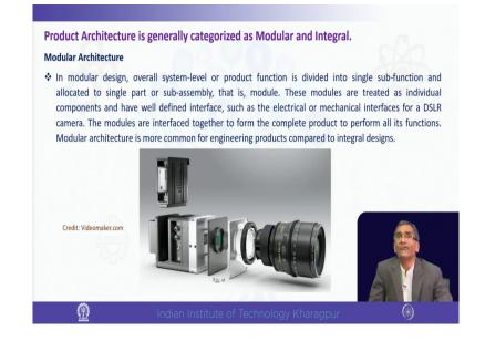
Now, we have touched on the modular and integral. There are two types of architecture one is modular, the other one is called integral. Modular that we have just understood from the earlier drawing, but here it is the image from which it is quite clear to you that how different modules are put together where the overall system level product function is divided into single sub function and allocated to a single part or sub assembly that is the module. We have already described that.
