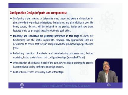
Now, after the architecture product architecture it is the configuration design of parts and components that is configuring a part means to determine what shape and general dimensions or sizes according to product architecture shape sizes the features there are different features also like say ribs, curves, holes etcetera are to be also provided.
