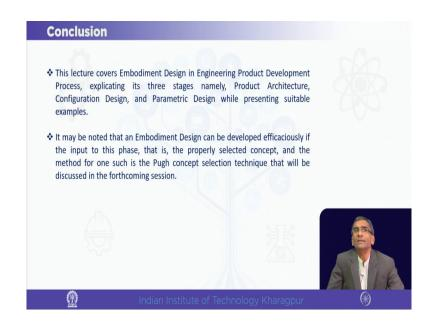
So, we discussed the three aspects of embodiment design that is product architecture, configuration design and parametric design here. It is important to know that to make the embodiment design this phase effective the correct selection of the concept is very important because that is the input.
