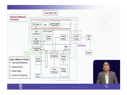
The next this diagram therefore, shows that we is in earlier case we said generate laser. Now, here we are saying CO 2 laser that is CO 2 laser process source is being used that is converged; that means, converging through a lens and then we said the focus the laser. Now, the laser how it is focused?
