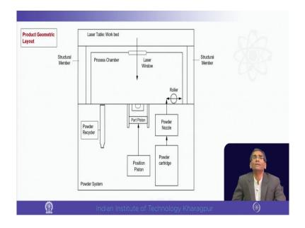
Now, this is the product geometrically out based on that architecture. On top it is the laser table, the structural member on both sides that process chamber, laser window all these things that we had seen. Now, this power recycler and power system all together is there this is the construction or geometric layout of the product.
