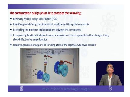
This is the example of configuration design how it is you know dimensions are provided etcetera that are done here. Reviewing product design specifications is done at this stage. Identifying and defining the dimensional envelope that is the within which space it would have to be manufactured total length, height, width kind of a thing like in I just I was talking about the rapid prototyping machine which has been called envelop within which it has to be produced.
